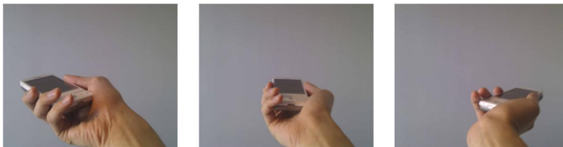
Figure 4-2. As shown from left to right, the phone subscriber can swing the smartphone to share draggable
