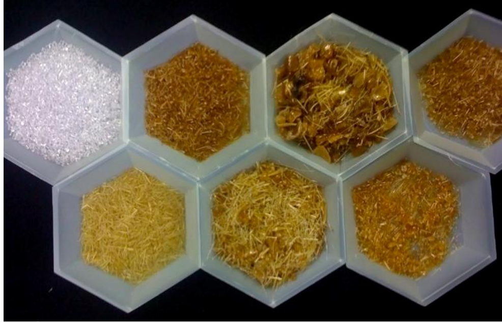
Figure 5.4 – Noticeable browning of composite samples after extrusion and pelletizing From LR: PC, 2% NCC-Alb / PC, 2% NCC-FP / PC (no antioxidant), 2% MF 40-10 / PC (dried), 2% MF 40-10 (solution), 2% NCC-FP / PC, and 2% UFC-100 / PC.
