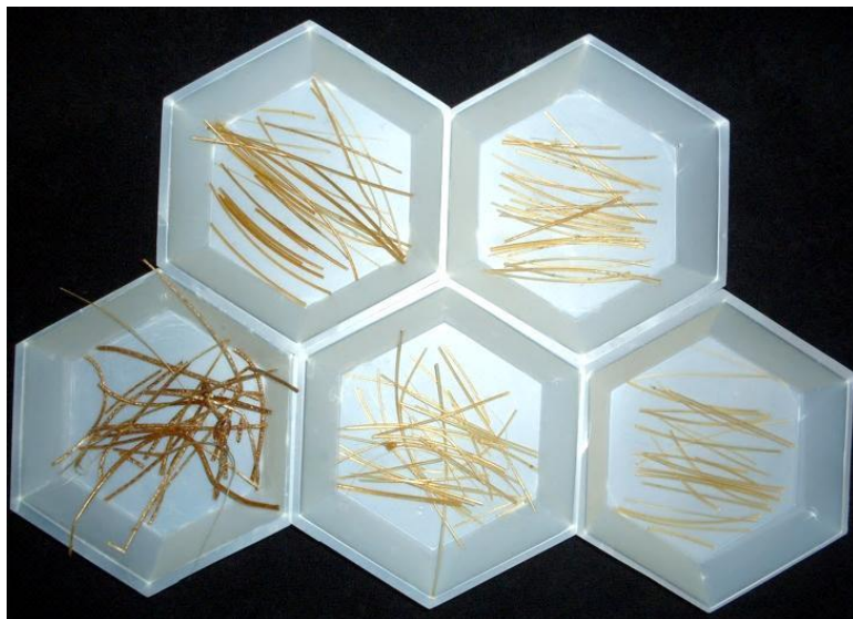
Figure 5.3 – Effect of extruder’s twin-screw rotation speed on polycarbonate discolouration over 50, 75, 100, 150, and 200 rpm
