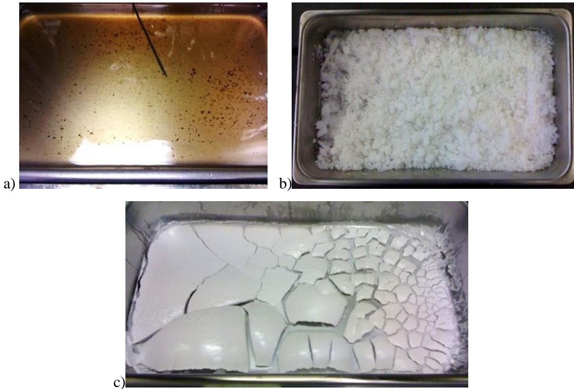
Figure 5.1 – Solution casting of composites a) 2% MF 40-10 / PC (dried), b) 2% NCC-Alb / PC, and c) 2% NCC-FP / PC
