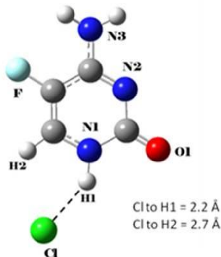
Figure 5.6: The lowest energy chloride-5-FC isomer, Cl-II, with relevant atoms labeled. For the purpose of reference, the same atom labels will be used when describing other isomers as well. Ionic hydrogen bonds are represented as black dotted lines and bond lengths are reported in Angstroms (Å).
