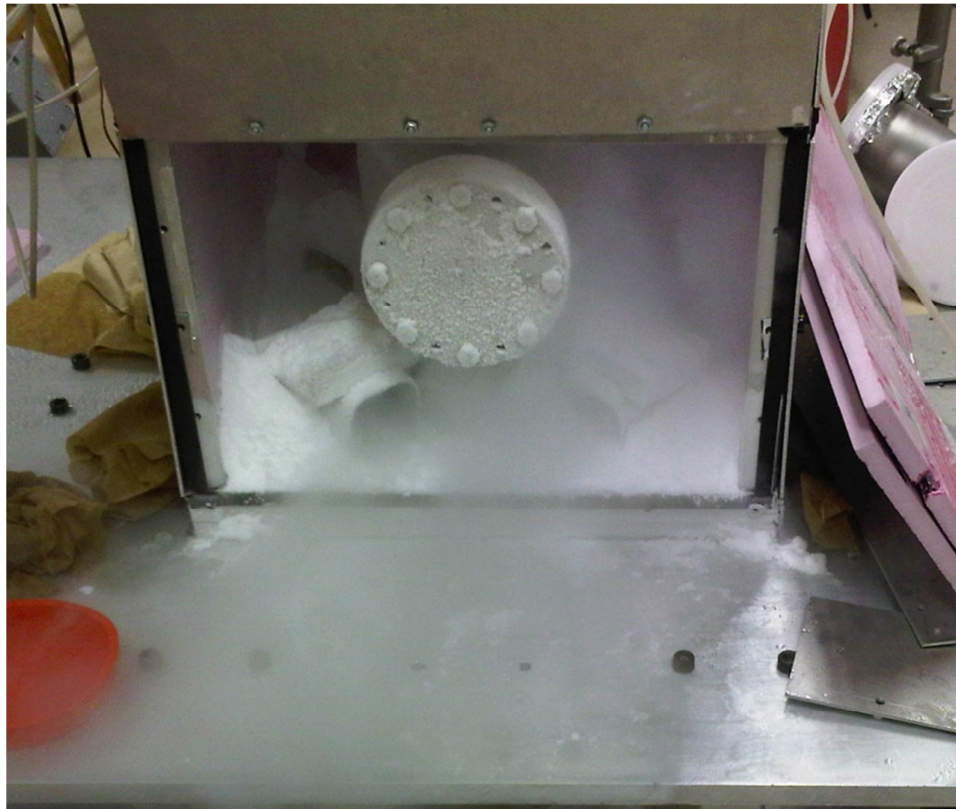
Photograph of the instrument inside the insulating cage. An access door is opened in order to remove dry ice after a low temperature experiment. A solid flange is used for low temperature tests instead of the sapphire viewport
