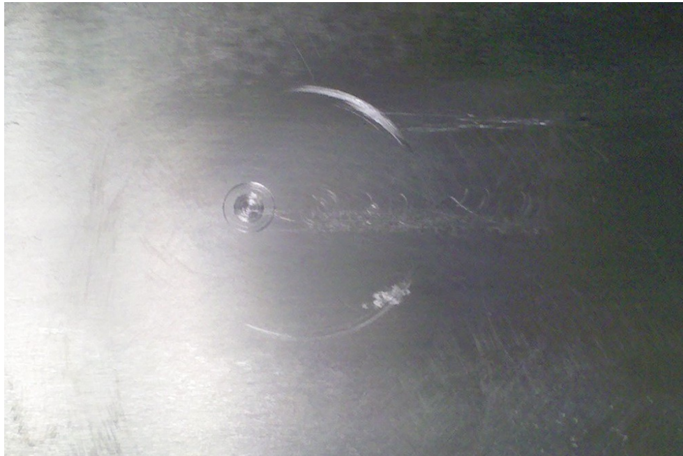
Figure 5.19: Large circular scratch pattern left by rotational experiments with aluminum specimen.
