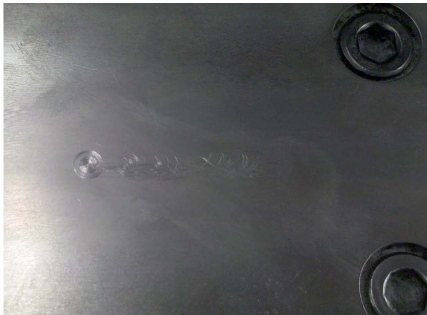
Figure 5.5: Wear to the titanium flat surface left by the 10 mm titanium specimen.
