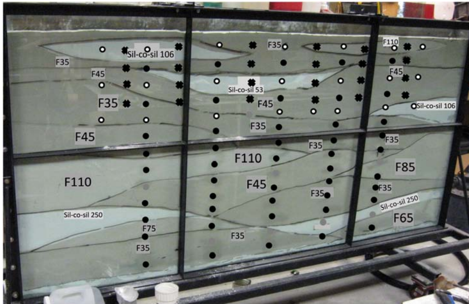
Figure 2.14. Photograph of the sandbox showing all sensor locations (● = pressure transducers; ● without pressure transducers; ○ = tensiometers; and x = water content sensors) and the various layers that were packed. Sensor locations are approximate. Numbers indicate what material type each layer is composed of.
