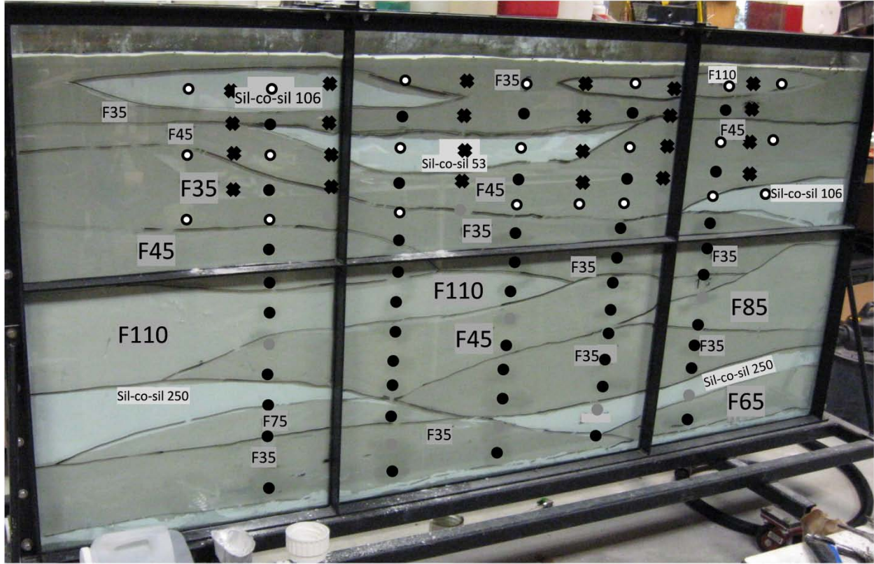
Figure C1: Photograph of the sandbox showing all sensor locations (● = pressure transducers; ● without pressure transducers; ○ = tensiometers; and x = water content sensors) and the various layers that were packed. Sensor locations are approximate.
