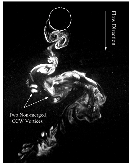
Figure 4.20 2P-like shedding pattern for case A1 ( U^* = 6.6 , z/L = 0.65 , \zeta = 0.007 , and U_c^* = 28.8 ).
