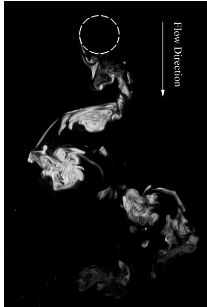
Figure 4.22 Flow visualization for case B1, ( U^* = 6.6 , z/L = 0.65 , \zeta = 0.01 , and U_c^* = 13.8 ).
