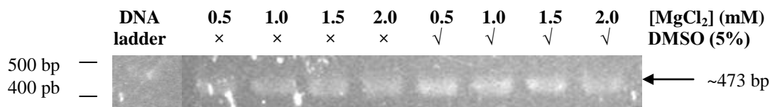
Figure 8.5: The agarose gel (1%) illustrates the PCR product of the putative lyase amplification using various concentrations of MgCl 2 with/without DMSO.
