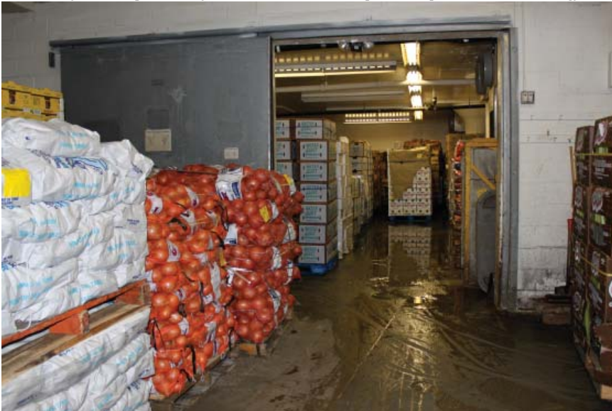
4.16 Lower level storage in tenant units are accessed by private elevator. Being below ground helps regulate temperature, as does the material choice - concrete block and poured concrete construction.
