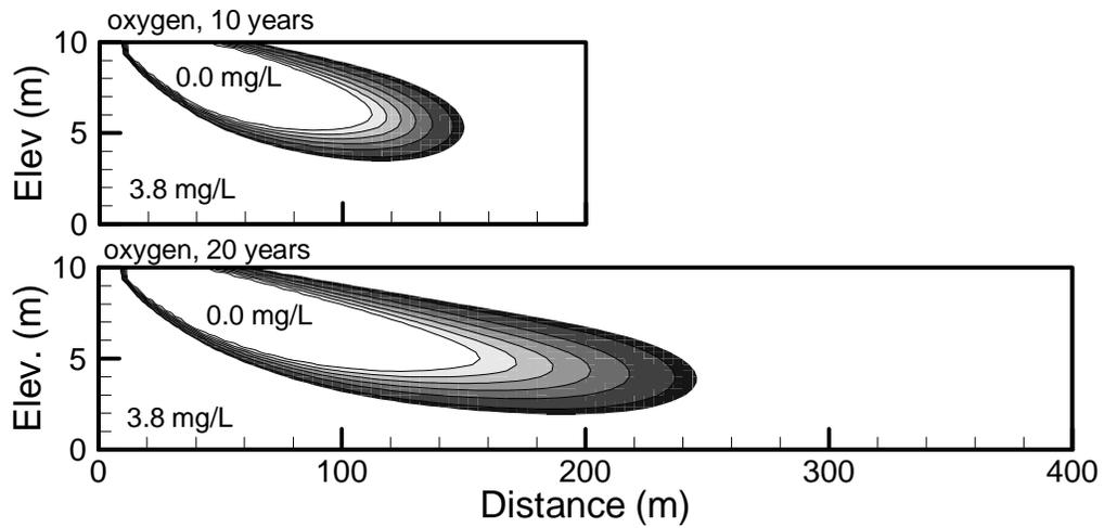
Figure 4.4: Simulated oxygen depletion plumes at 10 and 20 years.
