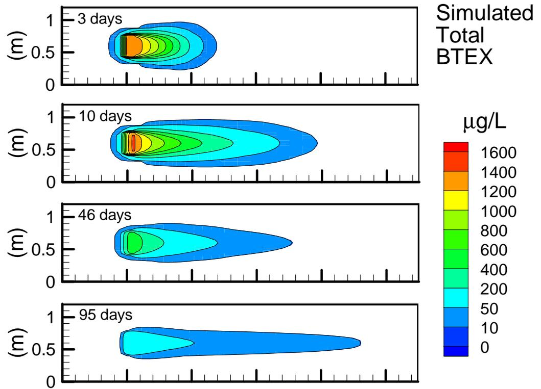
Figure 3.11: Simulated total BTEX plumes at 3, 10, 46 and 95 days. Plan view through source centre.
