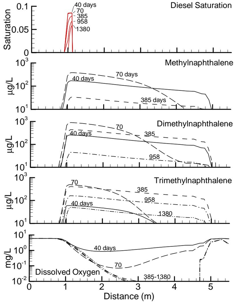
Figure 3.20: Simulated longitudinal profiles through the source centre showing diesel saturation, naphthalene concentrations and dissolved oxygen.
