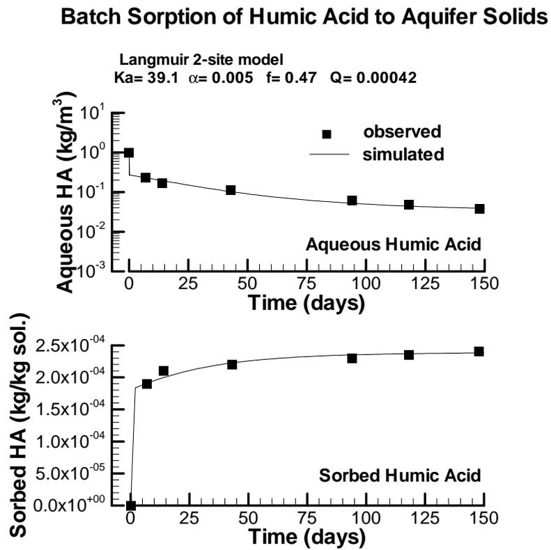
Figure 3.5: Observed vs. simulated transient sorption profile showing early equilibrium and late kinetic behaviour.
