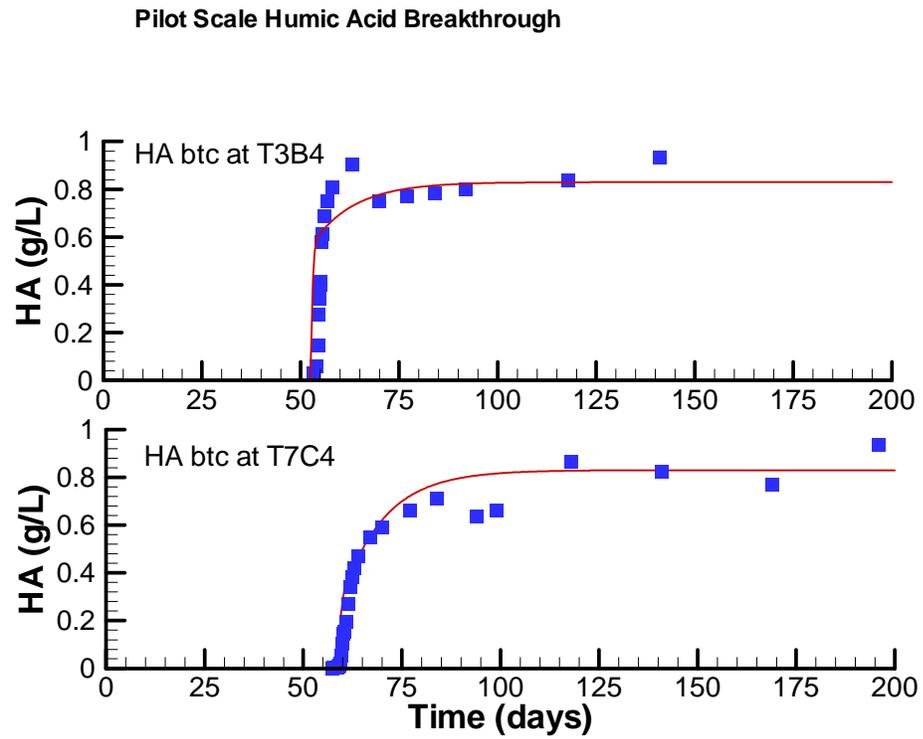
Figure 3.8: Simulated vs. observed breakthrough of the humic acid carrier in the pilot scale experiment at monitors T3B4 (top) and T7C4 (bottom).
