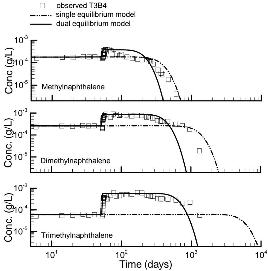
Figure 3.22: Observed vs. simulated breakthrough curves of the naphthalene components at T3B4 using single and dual-solubility equilibrium dissolution models.
