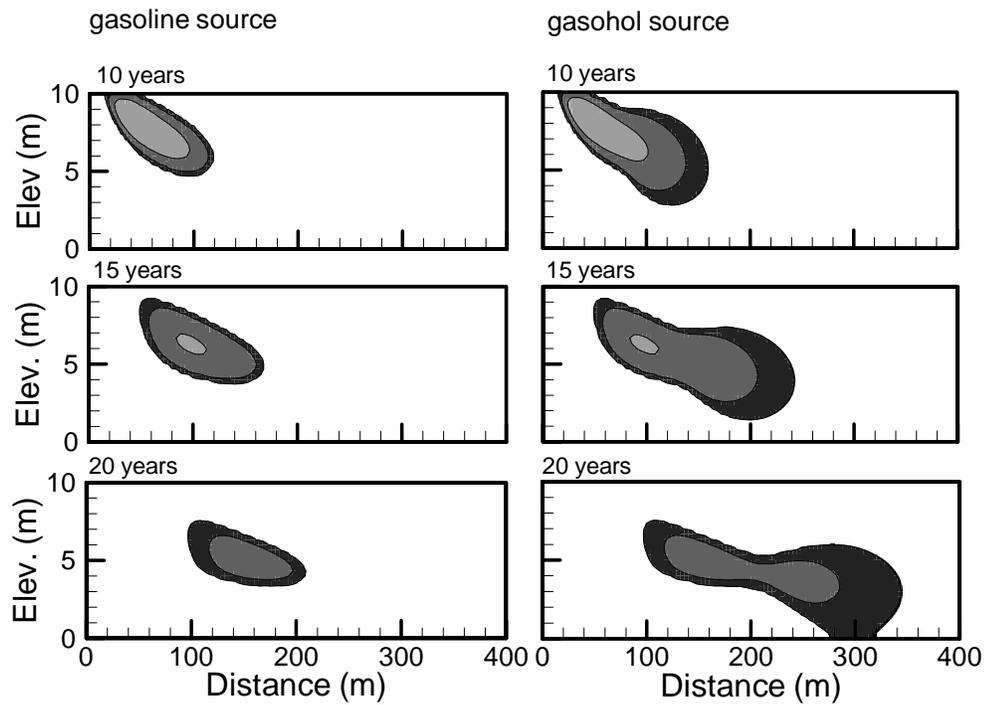
Figure 4.10: Simulated benzene plumes assuming a relatively lower background oxygen concentration of 2.0 mg/L.
