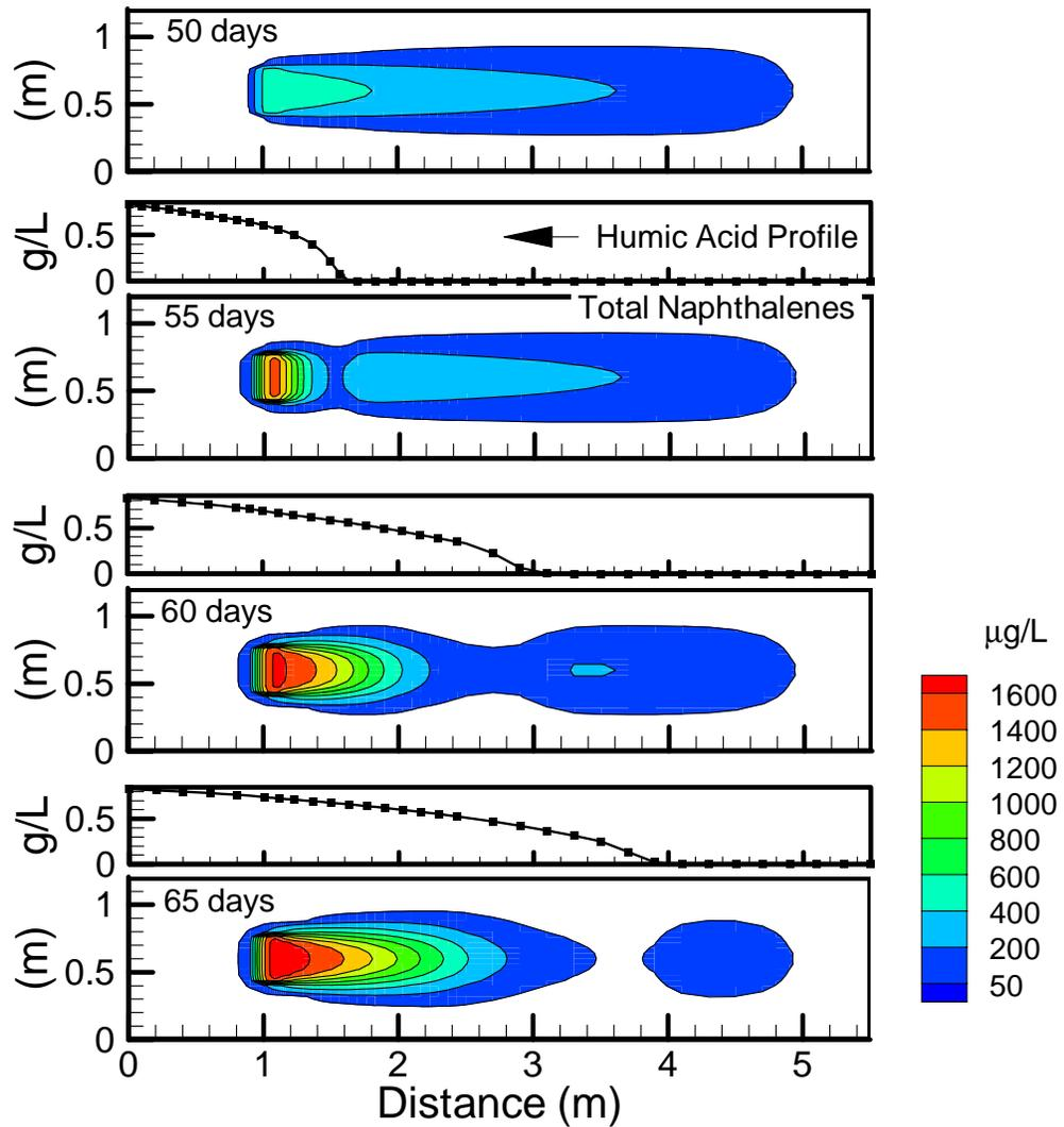
Figure 3.17: Simulated total methylnaphthalene plumes at 50-65 days showing corresponding humic acid profiles. Contour plots are plan view, located through the source centre.
