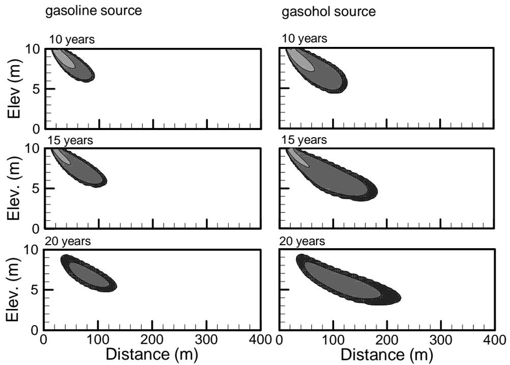
Figure 4.11: Multi-spill scenario: benzene plume evolution from gasoline (left) and gasohol (right) sources.
