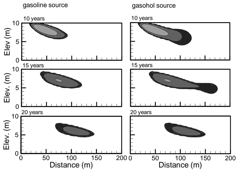
Figure 4.8: Simulated evolution of the benzene plume from a gasoline (left) and gasohol (right) source, assuming a relatively higher benzene retardation of 1.5.
