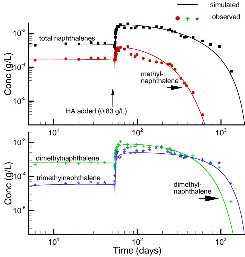
Figure 3.12: Observed vs. simulated breakthrough of the naphthalene components at monitor well T3B4 (immediately downgradient from the source).
