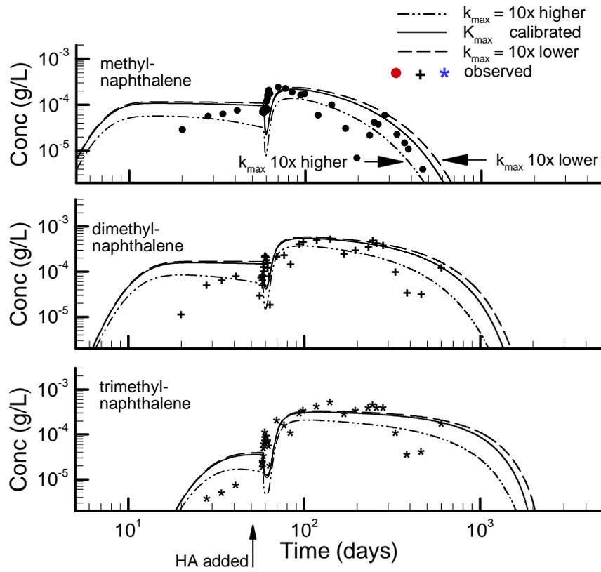
Figure 3.24: Breakthrough curves at T7C4 (1.5 m downgradient) showing effect of the maximum biodegradation rate for the naphthalenes.
