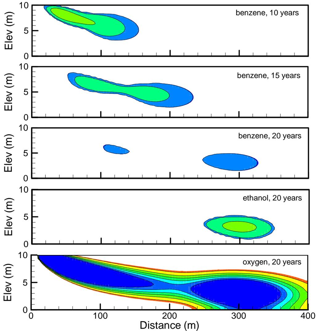
Figure 4.6: Simulated benzene plumes from the gasohol source at 10, 15 and 20 years. Also shown is the ethanol plume and dissolved oxygen depletion plume at 20 years. Benzene and ethanol concentration contours are 10, 100, 1000 ppb. Oxygen contours vary from a background of 3.8 mg/L to 0.0 mg/L within the gasoline and ethanol plumes.
