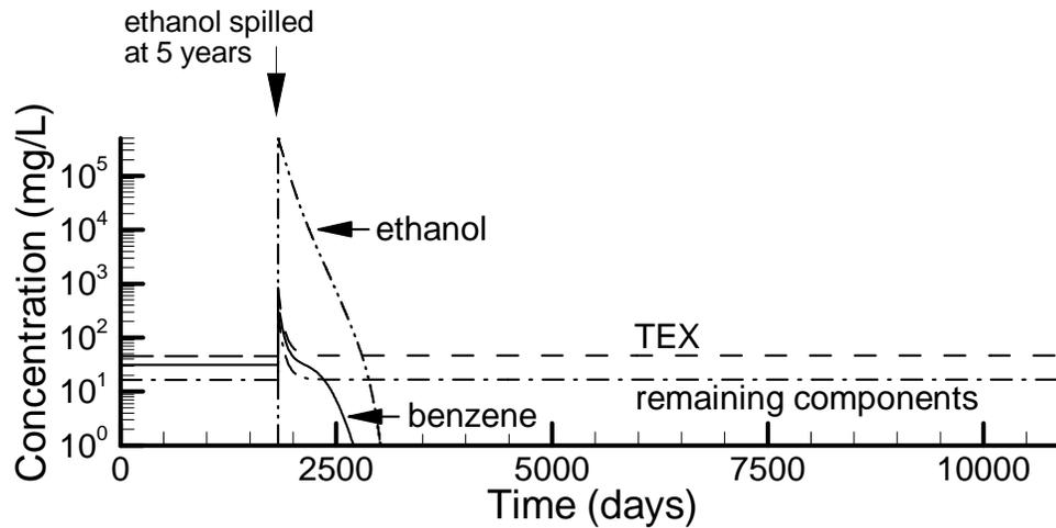
Figure 4.12: Simulated source concentrations for Conceptual Model 2: a pure ethanol spill at 5 years into an existing gasoline spill.
