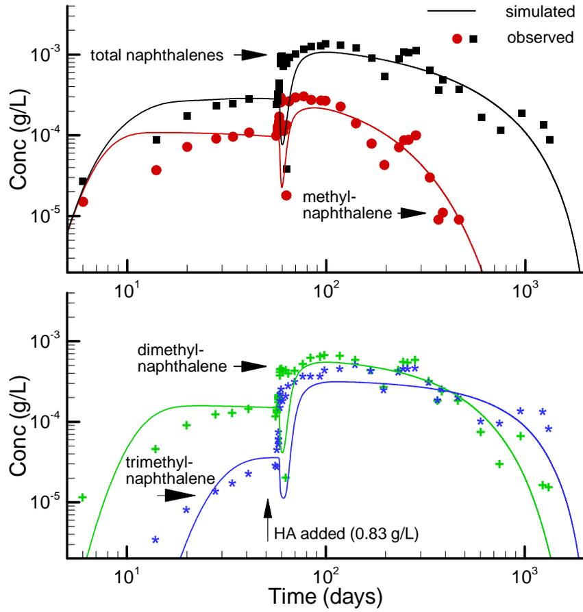
Figure 3.13: Observed vs. simulated breakthrough of the naphthalene components at monitor well T6B4 (1.2 m downgradient from the source).
