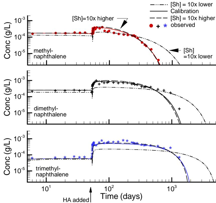
Figure 3.21: Sensitivity of naphthalene breakthrough to dissolution rate (Sherwood number), at monitor T3B4.
