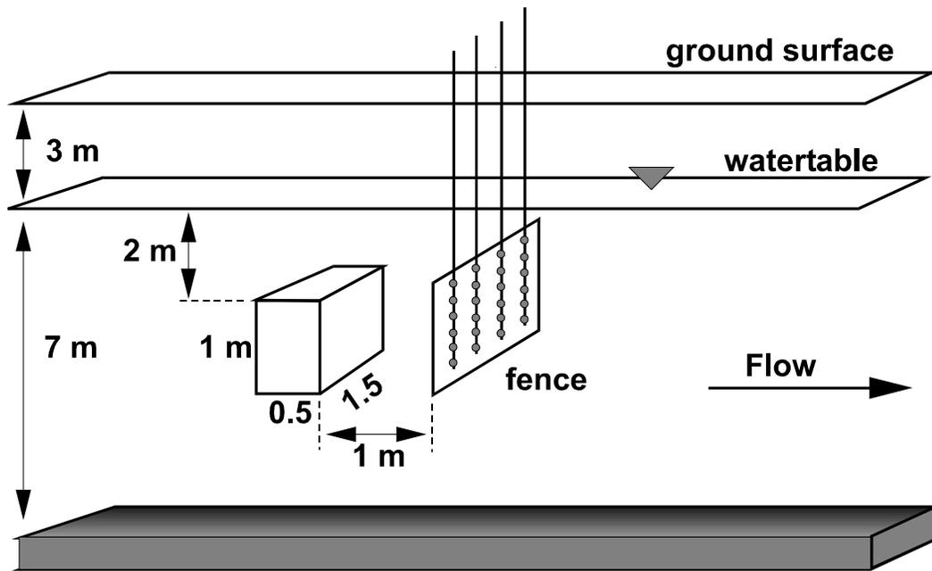
Figure 2.1: Layout of the Borden emplaced source experiment.
