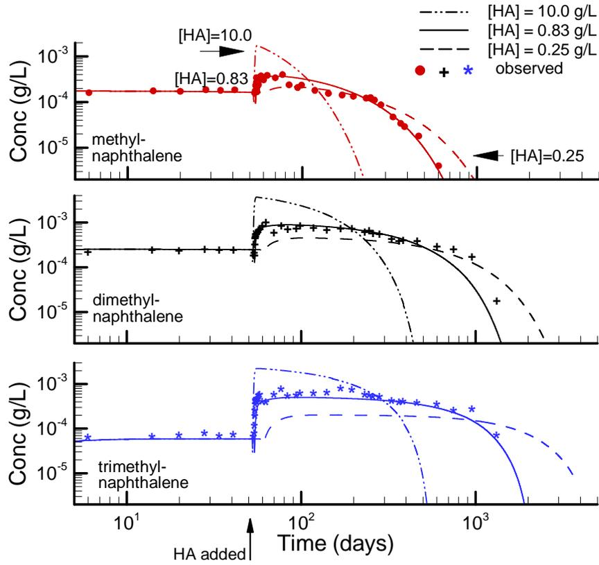
Figure 3.25: Breakthrough curves at T3B4 showing effect of humic acid concentration on enhanced dissolution of diesel fuel.
