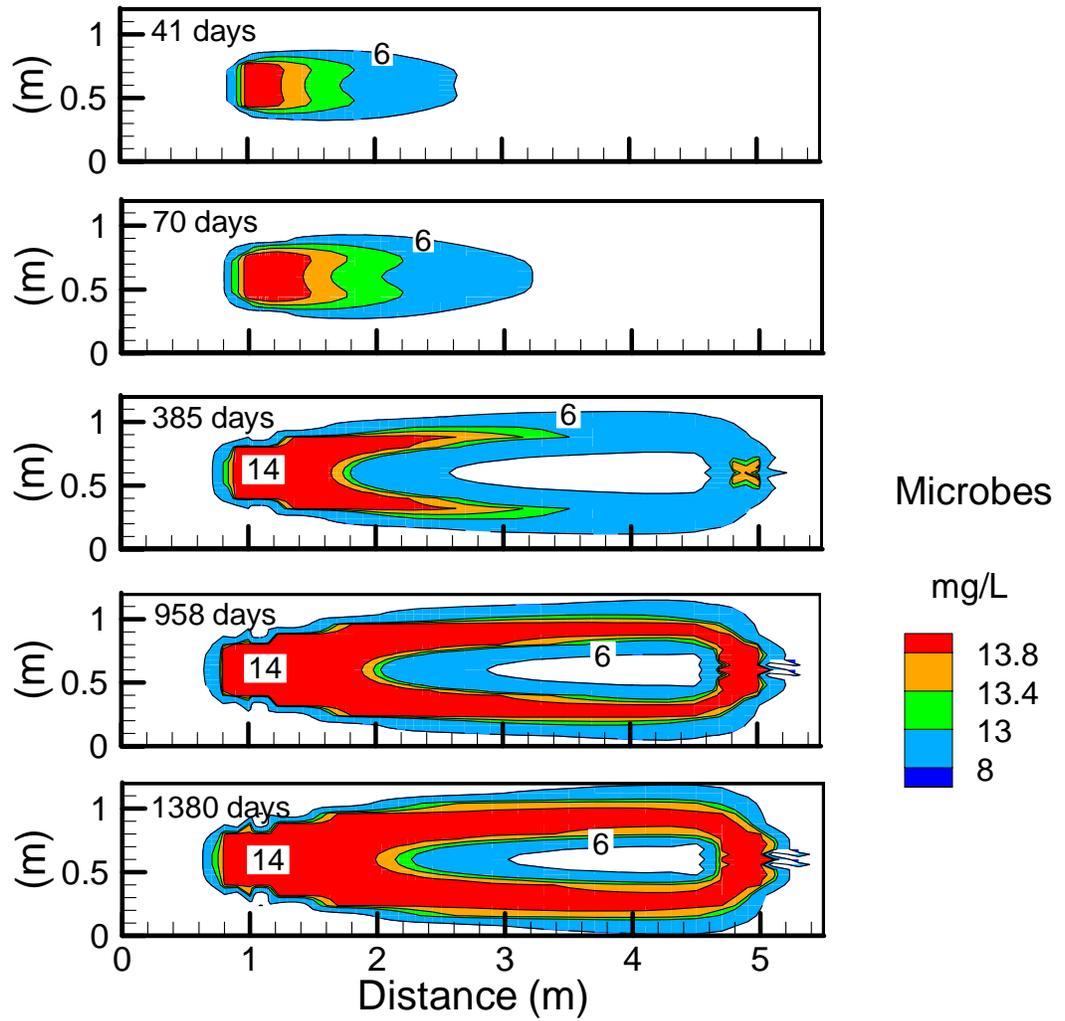
Figure 3.19: Simulated microbe concentrations within the pilot scale tank. Contour units are mg/L, plan view through source centre.
