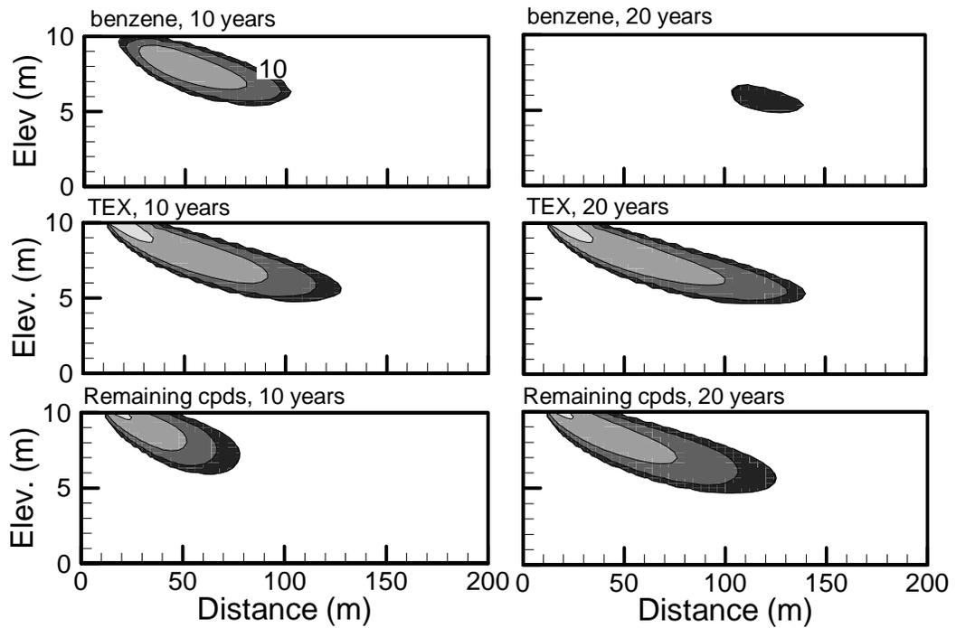
Figure 4.3: Simulated benzene, TEX and remaining component plumes from the base case gasoline source at 10 years (left) and 20 years (right). Contour intervals are 10, 100, 1000 and 10,000 ppb.
