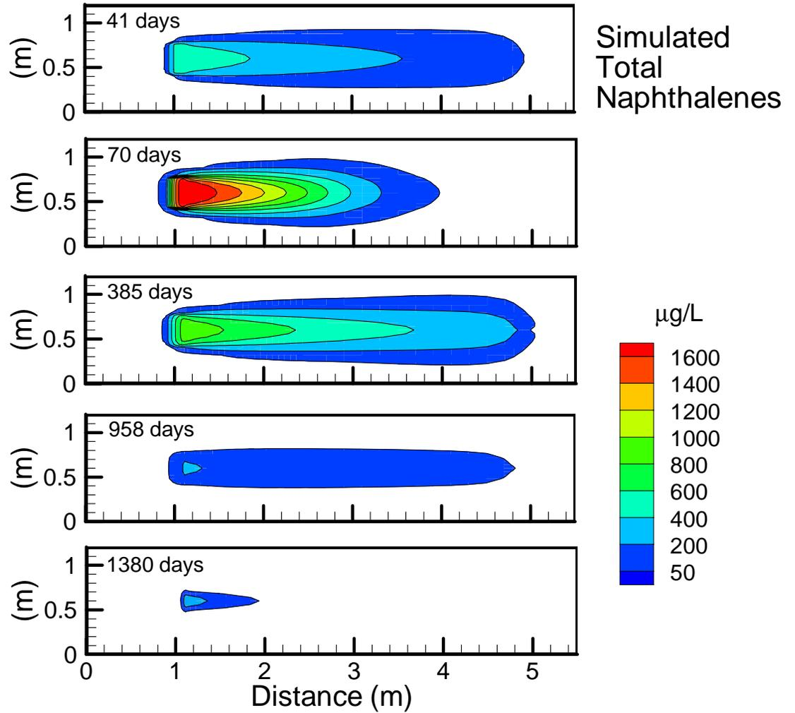
Figure 3.16: Simulated total methylnaphthalene plumes corresponding to observed times. Plan view through the source centre.
