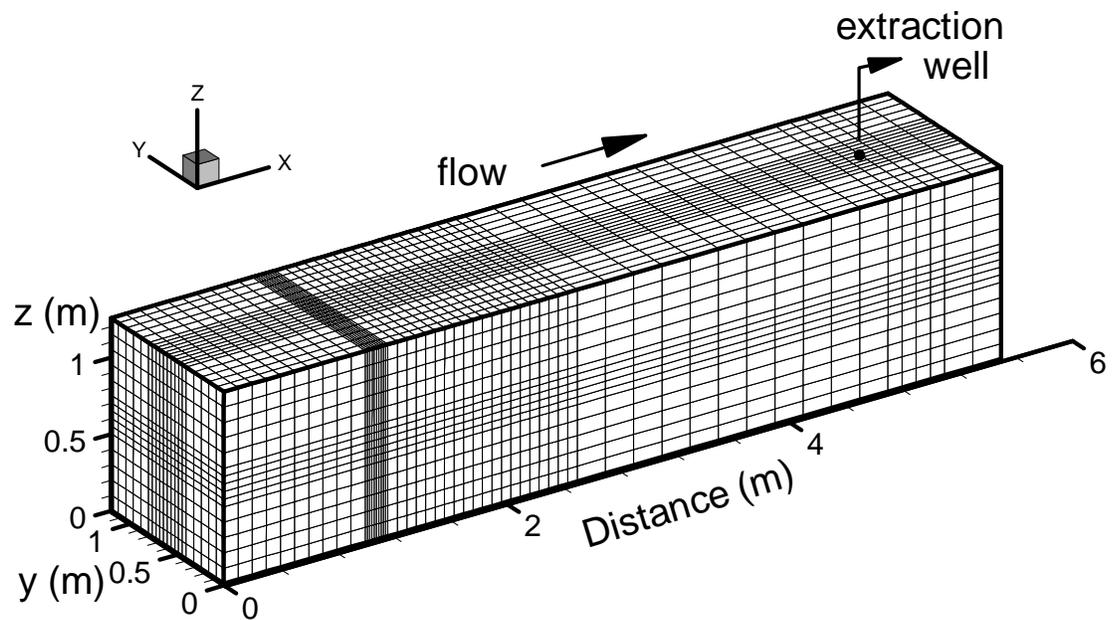
Figure 3.6: Outline of the 3D finite element mesh for the pilot scale model. The residual diesel source is located at the intersection of the fine-mesh areas, 1.0 m from the inflow boundary.
