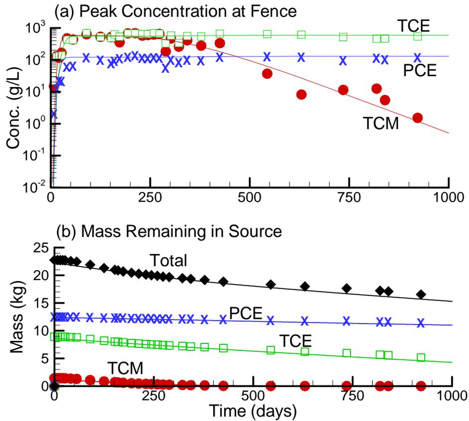
Figure 2.2: Observed (symbols) vs. simulated (lines) data for the emplaced source experiment: (a) peak concentrations at the 1-m fence, and (b) mass remaining in the source.
