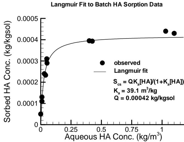
Figure 3.4: Observed vs. fitted Langmuir isotherm for lab batch sorption test of humic acid to winter sand (after Van Stempvoort et al., 2000).
