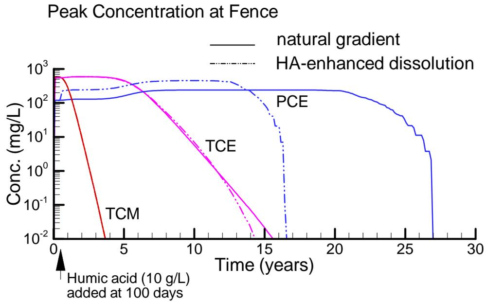
Figure 2.4: Comparison of long-term dissolution of the Borden source: Field condition (natural gradient) vs. HA-enhanced dissolution of PCE.
