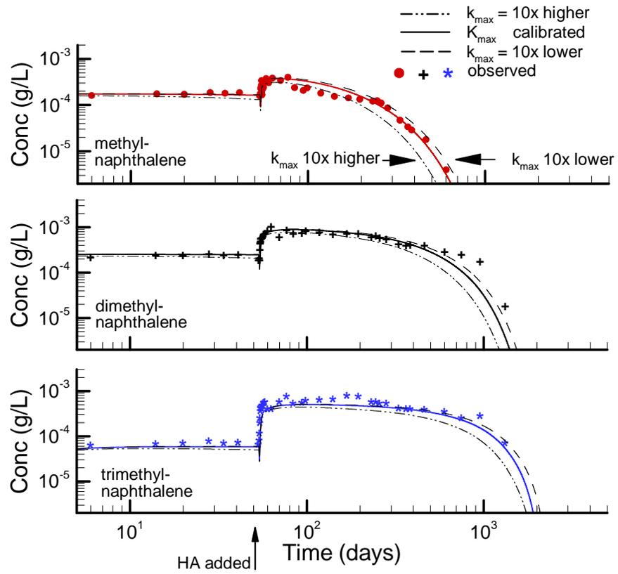
Figure 3.23: Breakthrough curves at T3B4 (immediately downgradient from the source) showing effect of the maximum biodegradation rate for the naphthalenes.
