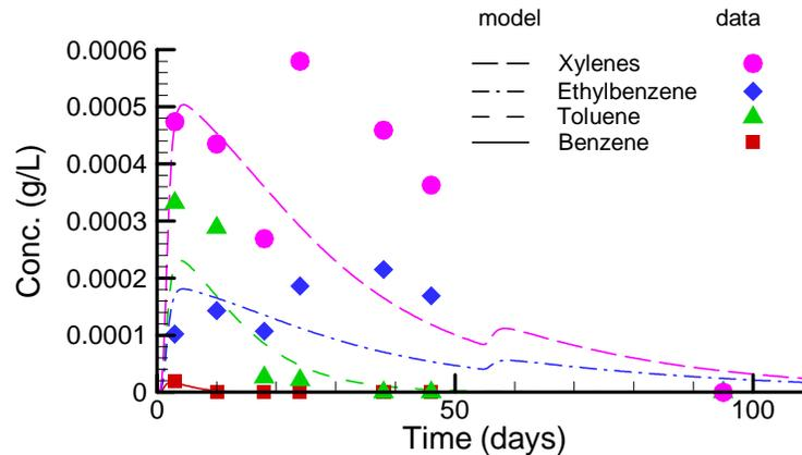
Figure 3.9: Simulated vs. observed BTEX concentrations at monitor T4M4.
