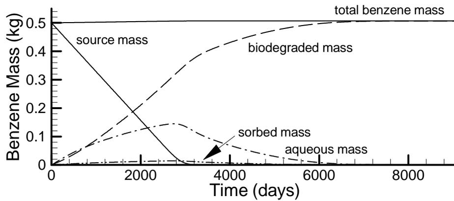
Figure 4.5: Simulated benzene mass distribution showing source mass depletion, mass lost to biodegradation and sorption, and aqueous plume mass.
