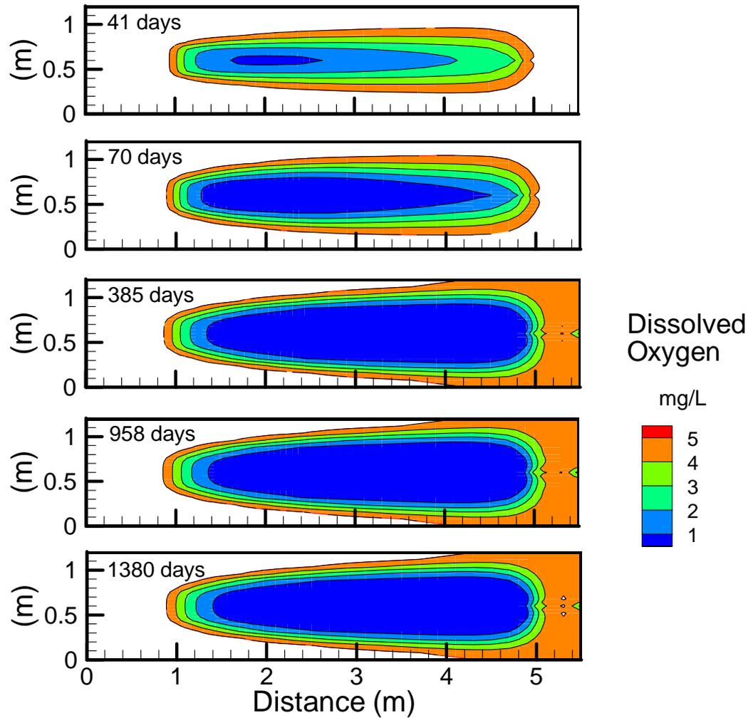
Figure 3.18: Simulated oxygen depletion plumes, caused by biodegradation of the diesel fuel components. The images represent a horizontal slice through the source centre. Contours are only flooded for depleted areas with less than the background concentration of 6 mg/L.
