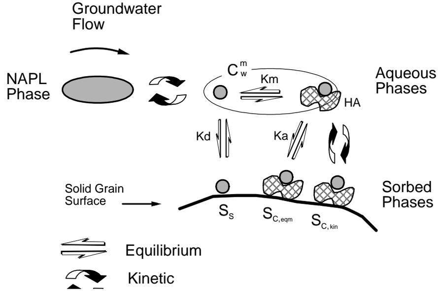
Figure 3.2: Conceptual model for NAPL dissolution and sorption to the organic carrier and solids. Here,  $C_w^m$  represents the aqueous pseudo-phase including both the free and carrier-bound dissolved organic.
