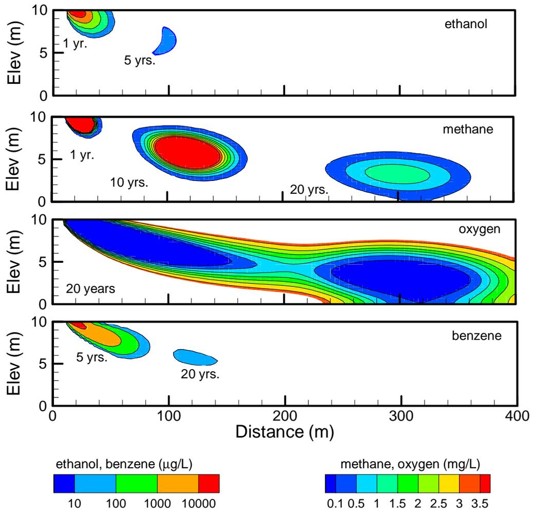
Figure 4.14: Simulated ethanol, methane, oxygen and benzene plumes: Conceptual Model 3.
