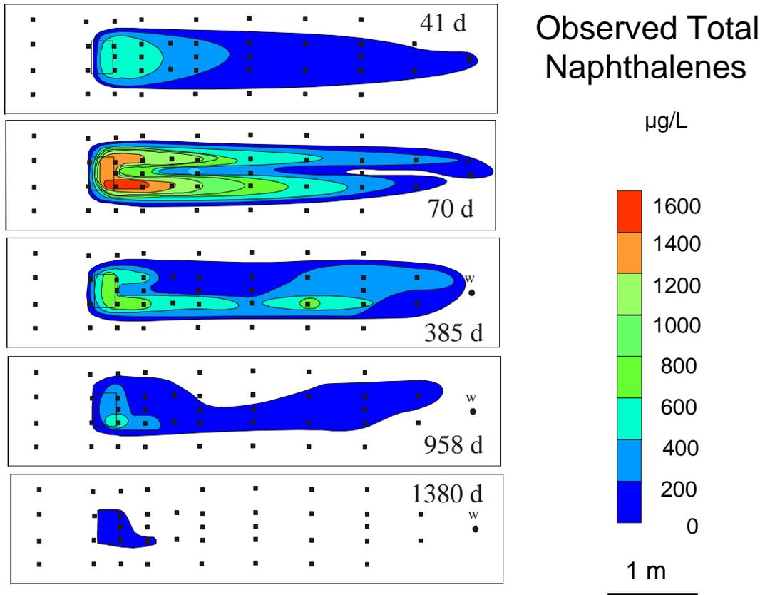
Figure 3.15: Observed total methyl-naphthalene plumes from the pilot scale experiment (plan view through source centre). After Van Stempvoort et al. (2000).
