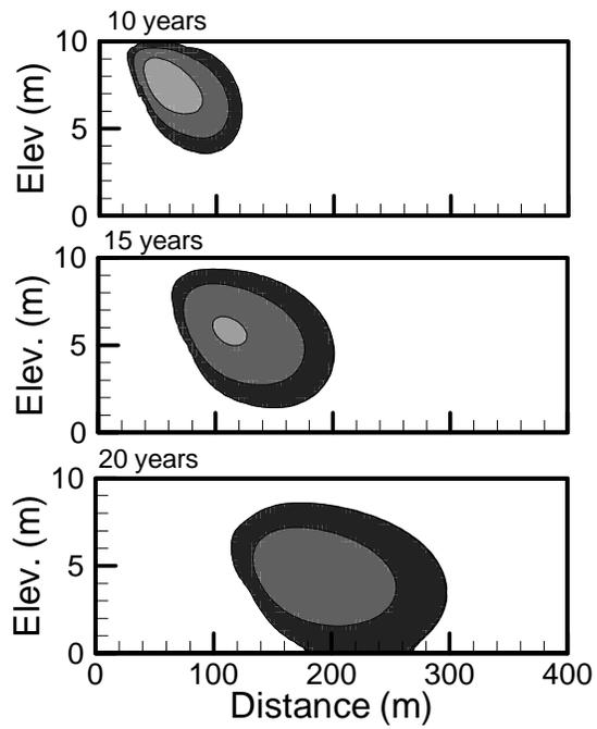
Figure 4.13: Benzene plumes from Conceptual Model 2: A pure ethanol spill into a 5-year gasoline plume. In this scenario, cosolvency effects are included.
