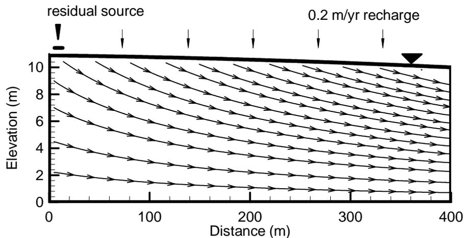
Figure 4.1: A vertical slice through the 3D steady state flow system assumed for the gasoline dissolution simulations. The residual source is located at the upper left.
