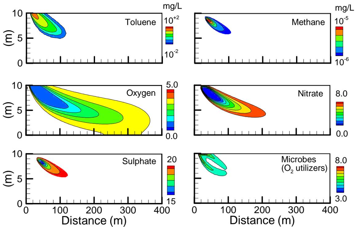
Figure 2.5: Simulated plumes, at 20 years, showing toluene and methane plumes, depletion of oxygen, nitrate and sulphate, and the growth of the oxygen-utilizing microbes. Electron acceptors are only plotted where they are depleted below their background levels. Vertical slice through a symmetric 3D system.
