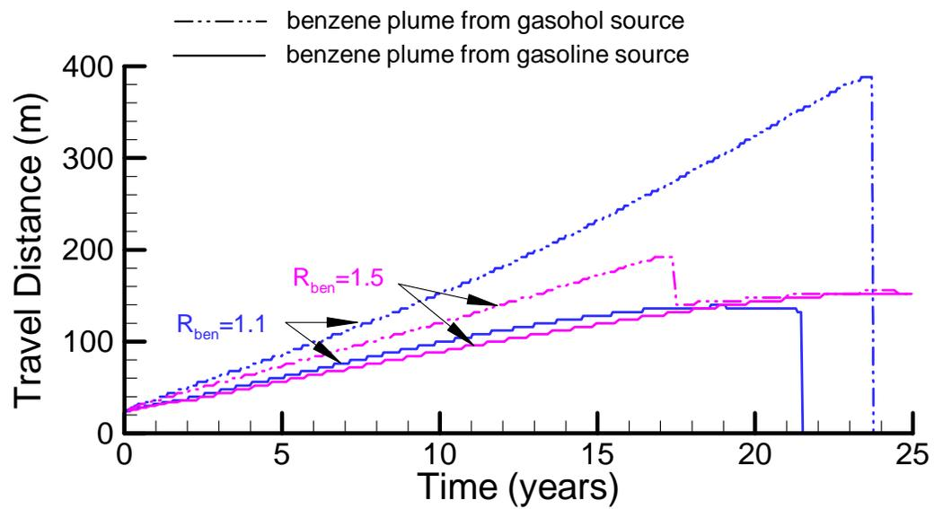
Figure 4.9: Simulated advance of the 10 ppb benzene contour from the gasoline and gasohol sources, comparing the effect of benzene retardation: base case ( $R=1.1$ ) and high-retardation scenario ( $R=1.5$ ).
