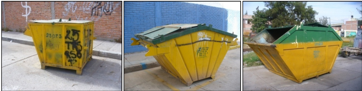
Figure 4.2: The three container sizes from smallest to largest (left to right): 1.3m 3 , 2.6m 3 , and 5.5m 3 .
