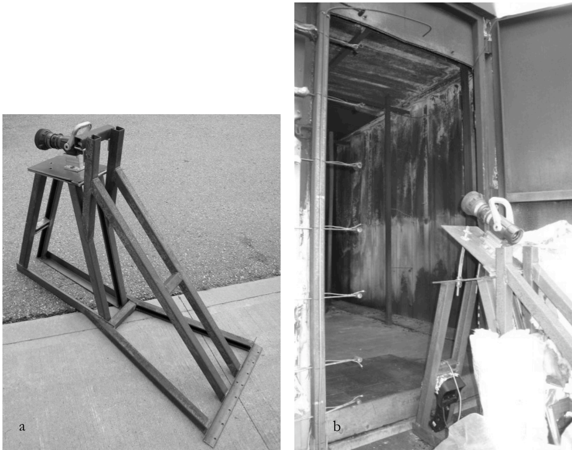
Figure 3.18. Suppression stand used in the experiments: (a) before instrumentation; (b) at the door.
