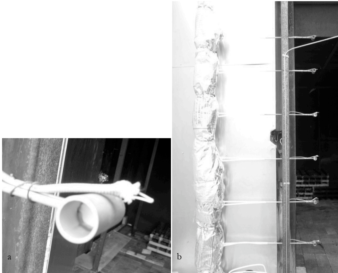
Figure 3.7. Bi-directional probe: (a) with attached thermocouple; (b) rake at the opening.
