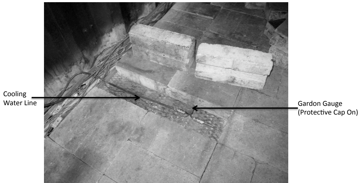
Figure 3.5. Uncovered floor mount heat flux gauge.
