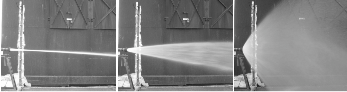
Figure 3.19. Nozzle flow patterns. L-R: straight stream, narrow fog, wide fog.
