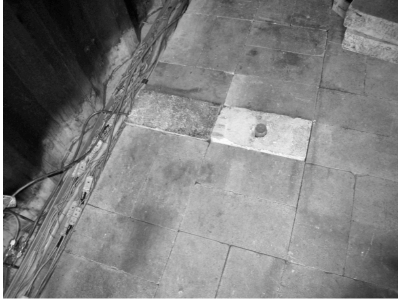
Figure 3.6. Covered floor mount heat flux gauge.
