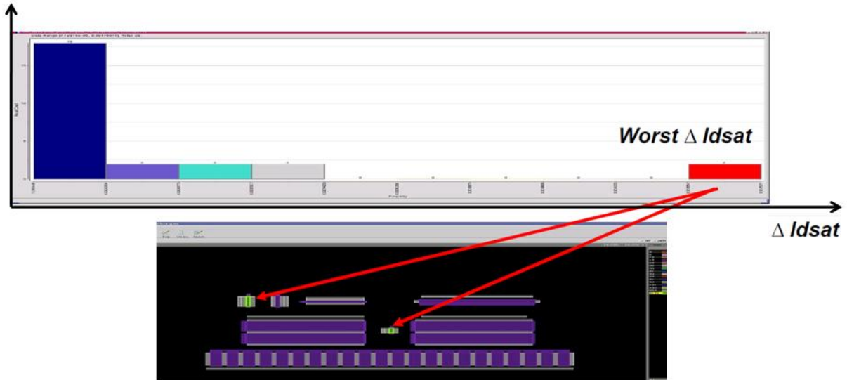
Figure 6.16: Histogram for worst case changes in saturation current I_{dsat} and pointing out most affected transistors in the tested layout design. [15]
