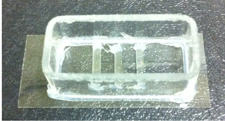
Figure 4-1: A 1 mm by 8 mm piece of microscope slide is cut and positioned in the center of a coverslip with medical grade silicone used at both sides. Polystyrene beads are used in the cell population cultured. The beads act as spacers between the coverslip and cut glass segment, which otherwise are held firmly together by the adhesive.
