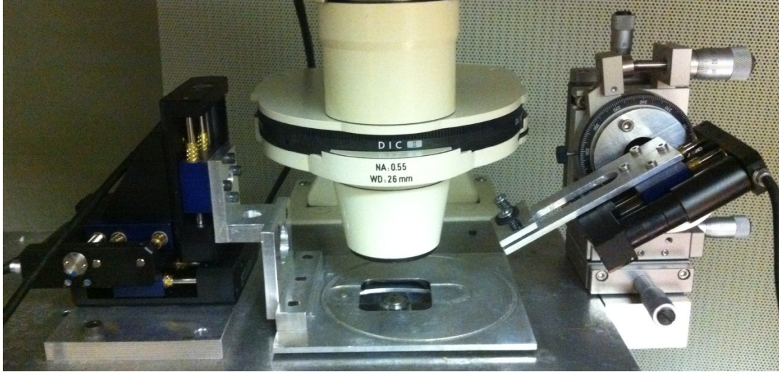
Figure 5-2: The complete three-axis robotic stage (x,y and z-axis) is on the left and the micropipette positioning system (or w-axis) is on the right.
