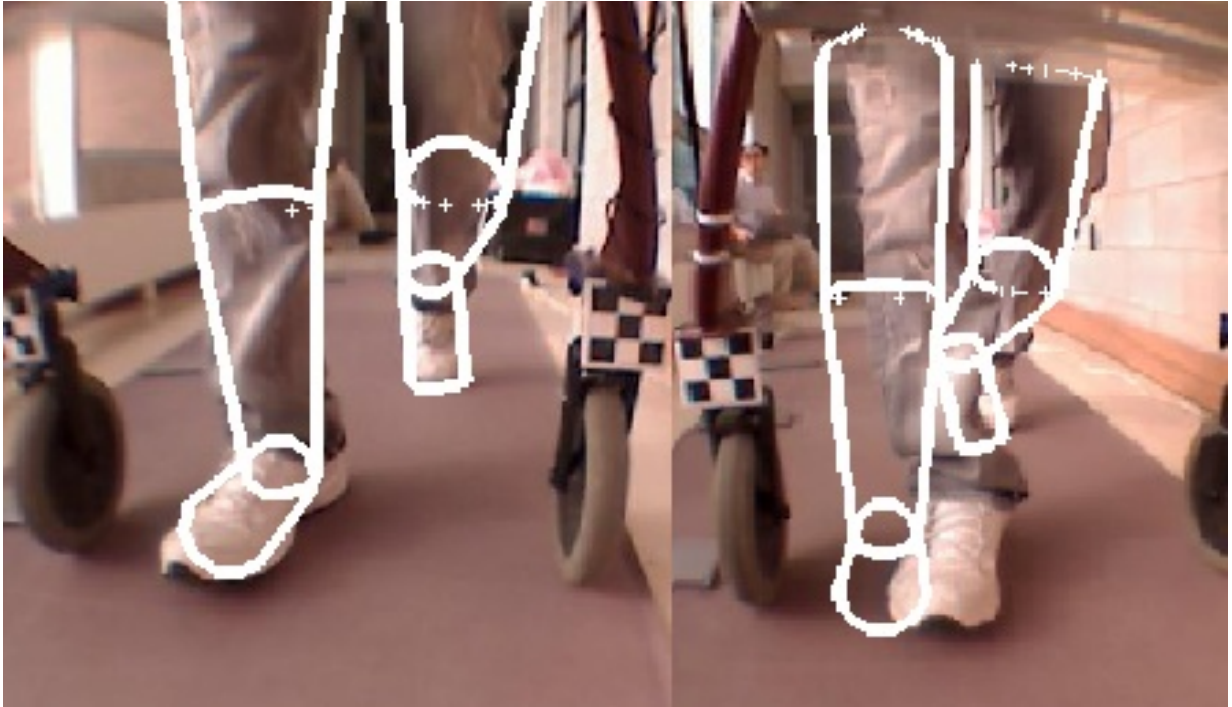
Figure 3.5: Depth error reflected in a binocular setup
