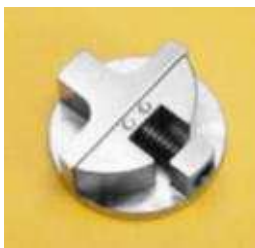
Figure 3-6 AFM sample holder used for the membrane fibers (Bruker AFM Probes)
