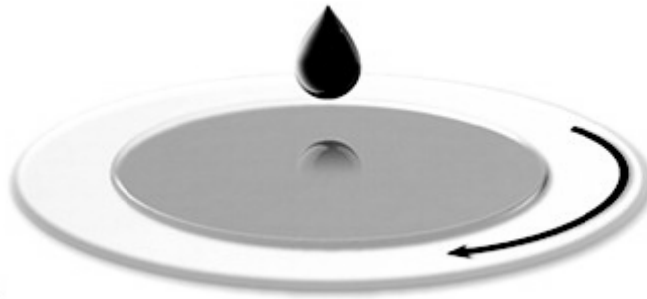
Figure 2.5 - Schematic image of spin coating process [42]
