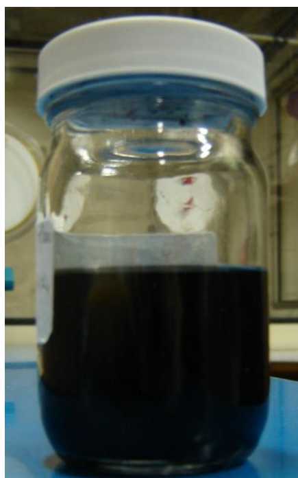
Figure 3.3 - Optical image of functionalized SWCNT suspension two months after preparation
