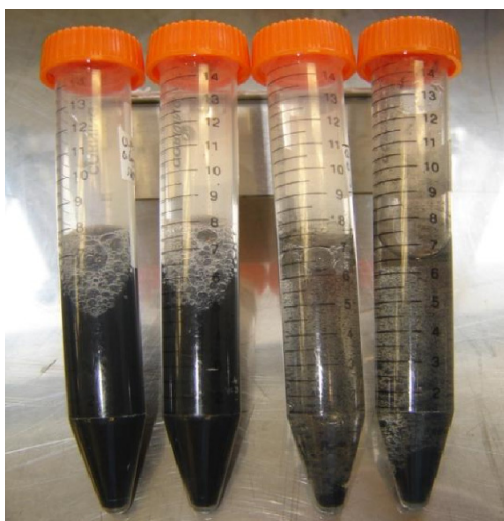
Figure 3.1 – SWCNTs dispersed in H 2 O using decreasing concentrations of SDS
