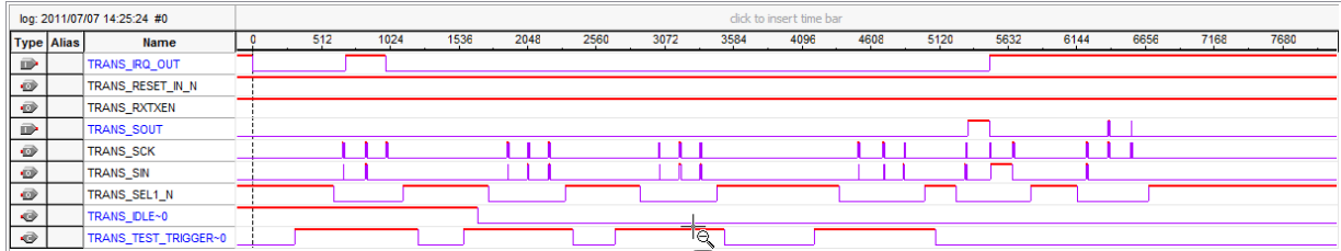
Figure 5.4: SignalTap II Output showing successful stream transmission
