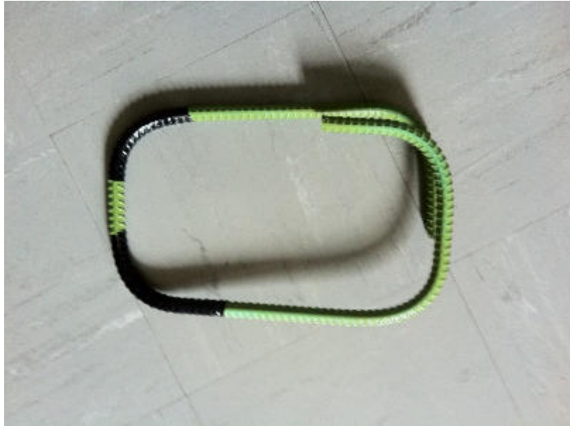
Figure 3-6 Epoxy coated stirrups with electrical tape at the corner
