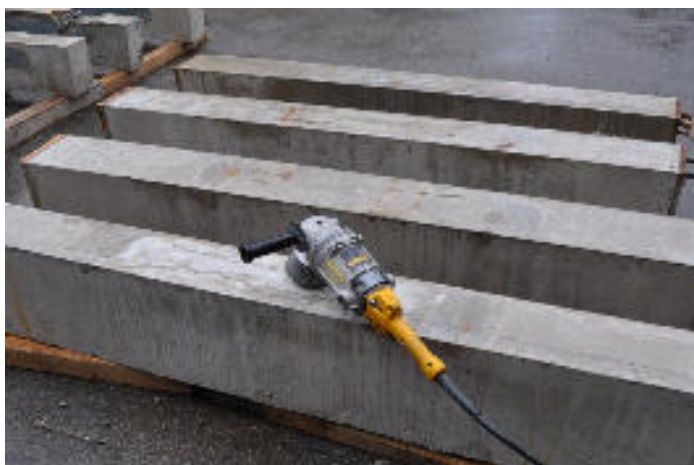
Figure 3-14 The specimen surface before and after cleaning
