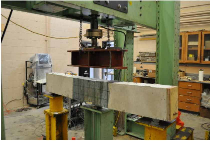
Figure 3-13 CFRP repair scheme
