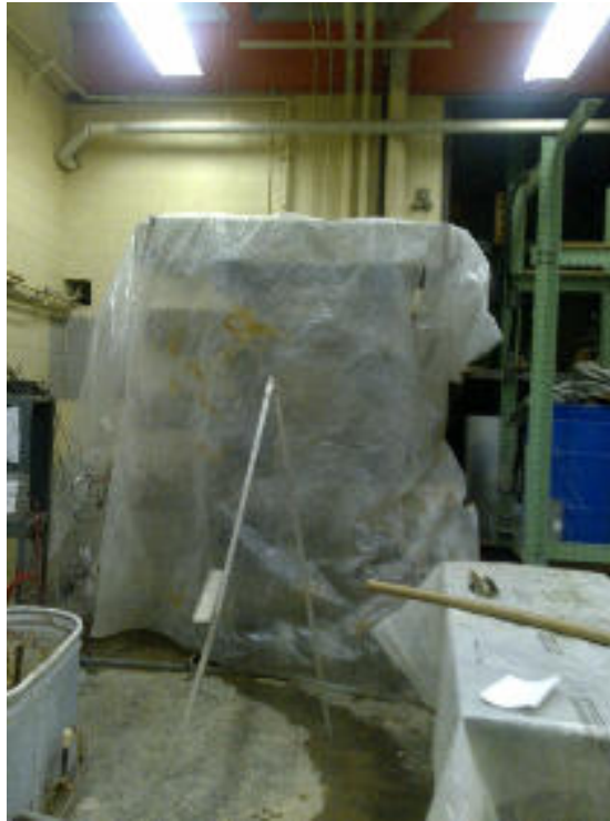
b) Corrosion chamber with beams
