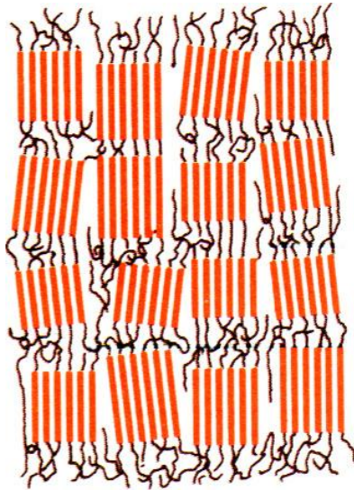
Figure 1.21 - Semi-crystalline microstructure, oriented in the loading direction (Winkler, 2009)
