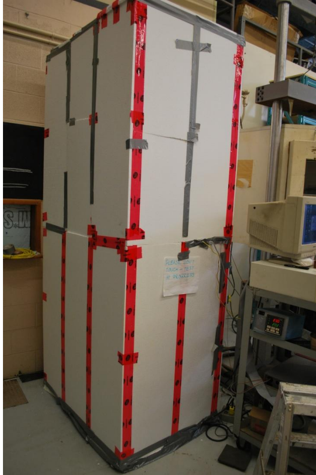
Figure 2.4 - Insulation enclosure for test frame
