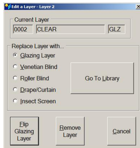
Figure A.2: The Edit Layer dialogue allows you to change or delete the selected layer.
