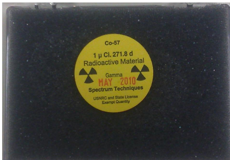
Figure 52. Co 57 gamma source used to generate 122 keV photons.
