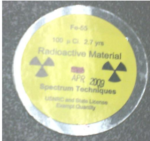
Figure 50. Fe 55 gamma source used to generate 6 keV photons.
