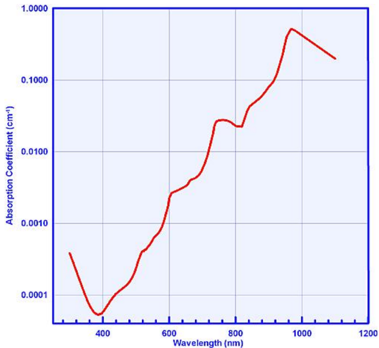
Figure 2.6: This plot shows the absorption of light in water as a function of the wavelength of the light. Light around 400nm has the lowest absorption / greatest transmissivity through the water.[28]
