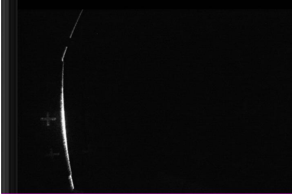
Figure 3.1: Picture captured with the CCD image sensor showing the laser line in the image.
