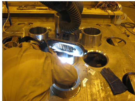
(b) Stage 2 Welding on Shell OD Side
