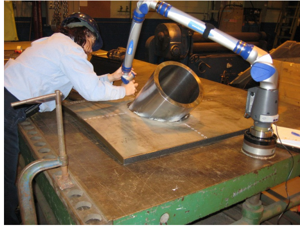
Figure 3-8 Single Nozzle Weld Distortion Measurement with FARO-ARM Platinum
