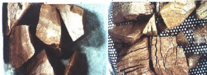
Figure 5: Aggregates before (left) and after (right) soundness test [PI 2007a].
