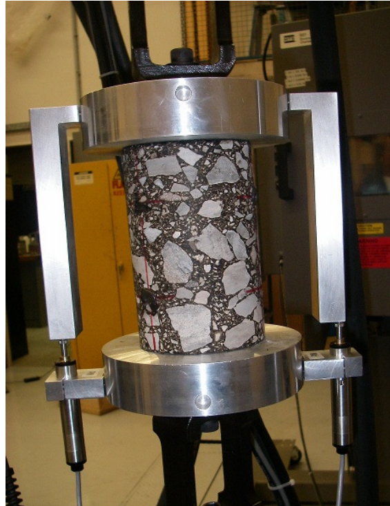
Figure 8: Dynamic Modulus Test Setup, CPATT Laboratory
