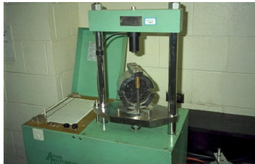
Figure 2: Marshall Stability and Flow test [Hoffman 2008b]
