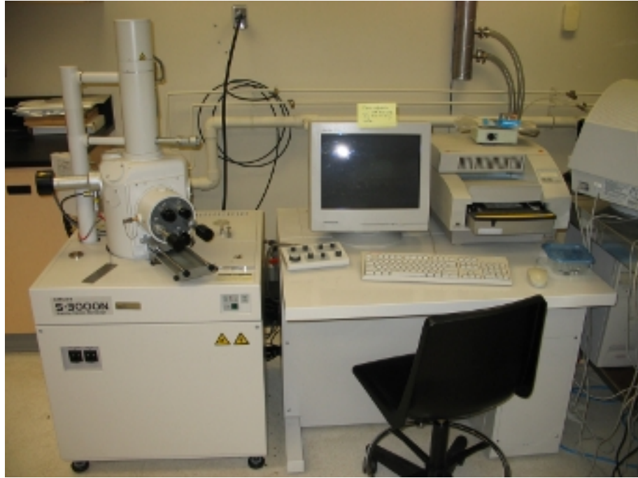
Figure 5.3: Hitachi S-3000N scanning electron microscope utilized to characterize the phononic band gap quasi-crystal and reference devices described in Table 3.1 fabricated in the SOIMUMPs [47].
