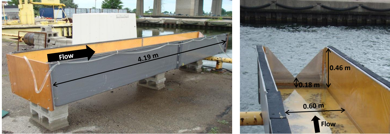
Figure 2.1: Design and dimensions of the weir box.
