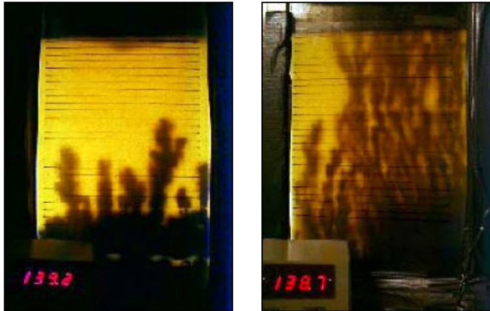
Figure 2.3 – Photographs of viscous fingering developing in two phase systems. Left: No pressure pulsing. Right: Pressure Pulsing (Davidson et al 1999)
