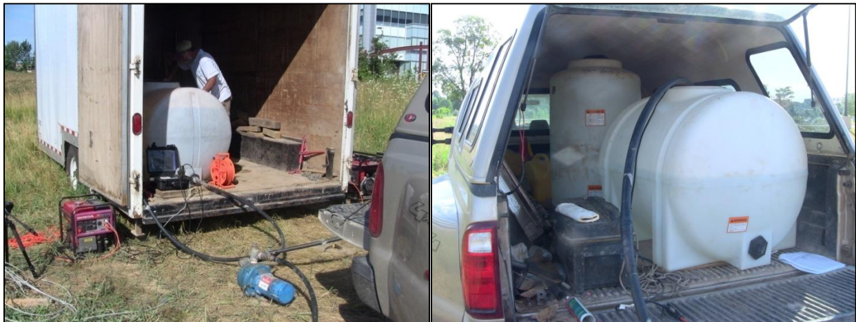
Holding tanks used to store tracer solution at ground surface (3250 L capacity)
