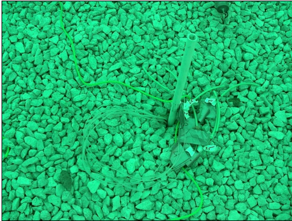
Multilevel well-head, including adaptor tubing used to connect syringes
