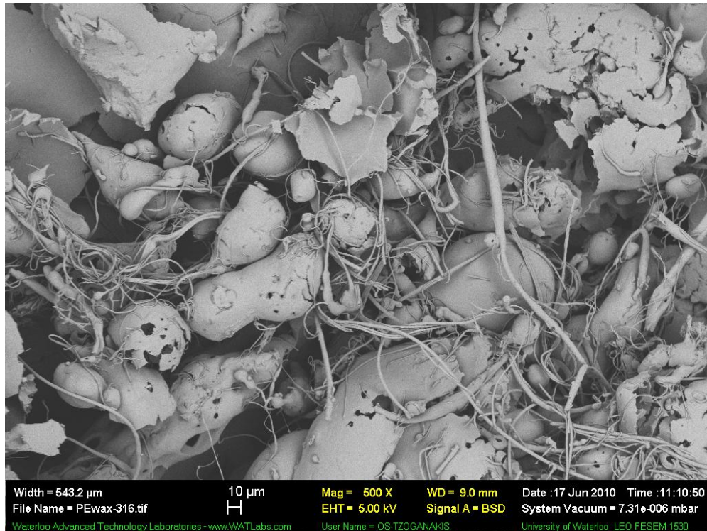
Figure 4.11: SEM Images of Particles Produced at Different CO 2 Feed Rate at 500X Magnification (Polymer Feed Rate= 55 g/min, Screw Speed = 50 rpm, Nozzle Temperature = 140°C): (a) 45 ml/min and (b) 55 ml/min
