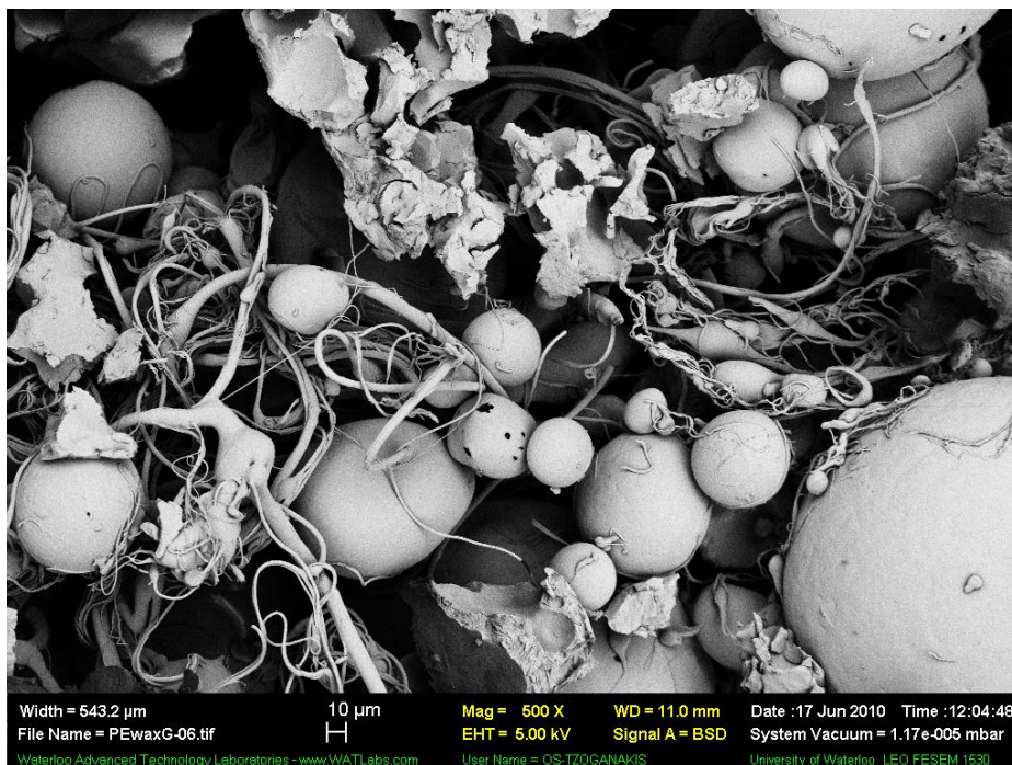
Figure 0.18: SEM Images of Particles Produced at Polymer Feed Rate= 26 g/min, CO 2 Feed Rate =25 ml/min, Screw Speed =50 rpm, and Nozzle Temperature =180°C
