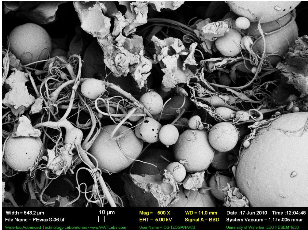
Figure 4.10: SEM Images of Particles Produced at Different Polymer Feed Rates at Nozzle Temperatures 180°C (CO 2 Feed Rate = 25 ml/min, Screw Speed = 50 rpm): (a) 13 g/min and (b) 26 g/min
