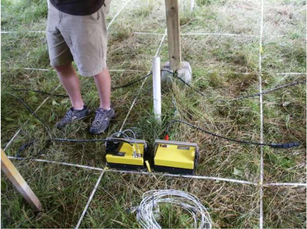
Figure 2.5 – GPR antennas positioned in the parallel orientation.
