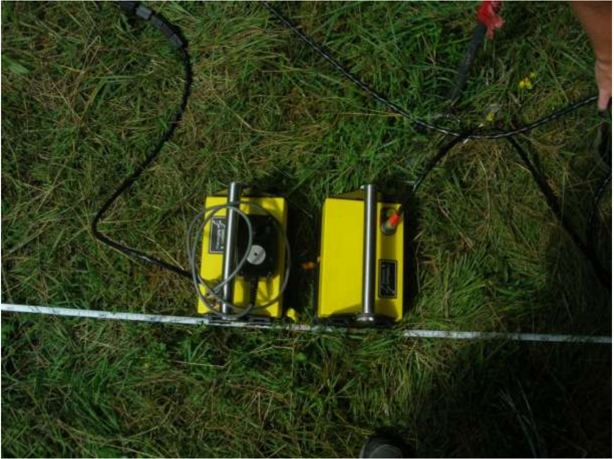
Figure 2.4 – GPR antennas positioned in the perpendicular orientation.
