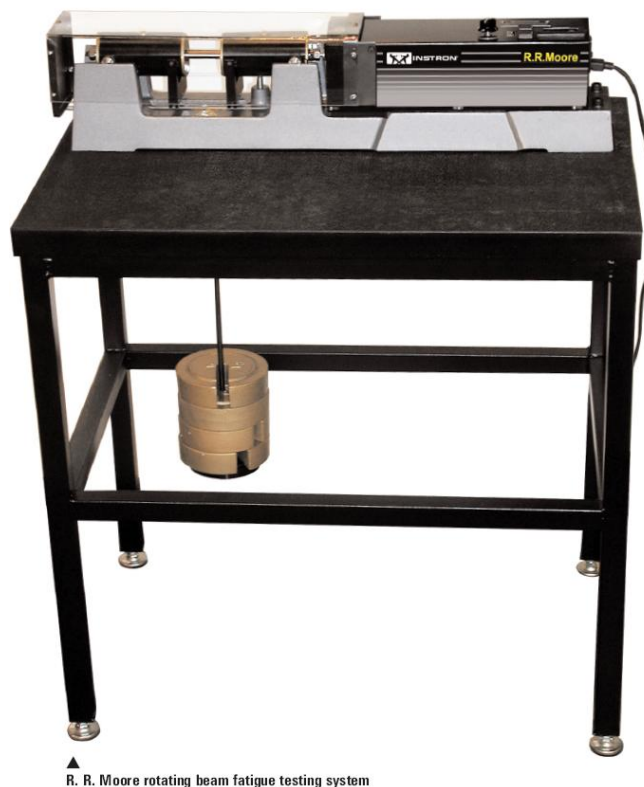
Figure 68- Rotating Bending Machine Used for Fatigue tests [52]
