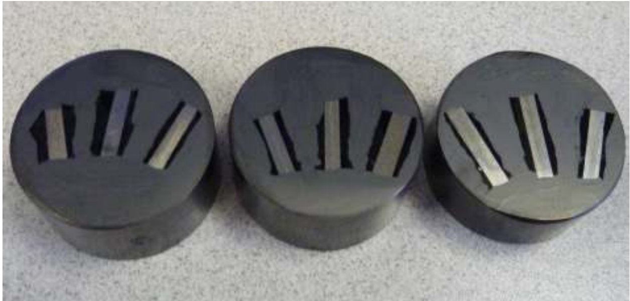
Figure 19 - Samples from Experiments 1 through 9 from left to right, mounted in an EpoFix cold mount and covered in colloidal graphite
