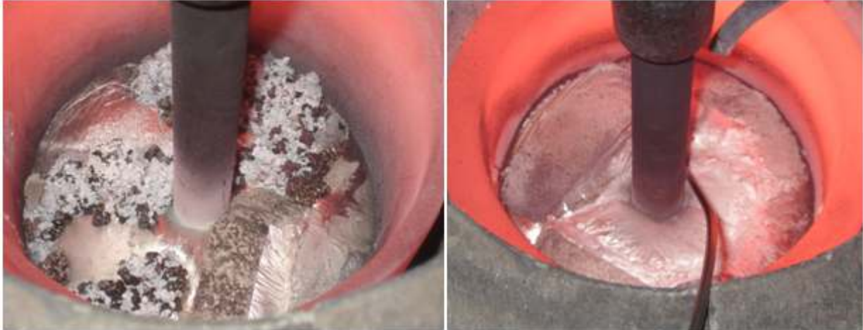
Figure 64 - Difference of Melt Pool with (Right) and without (Left) protective gas shielding
