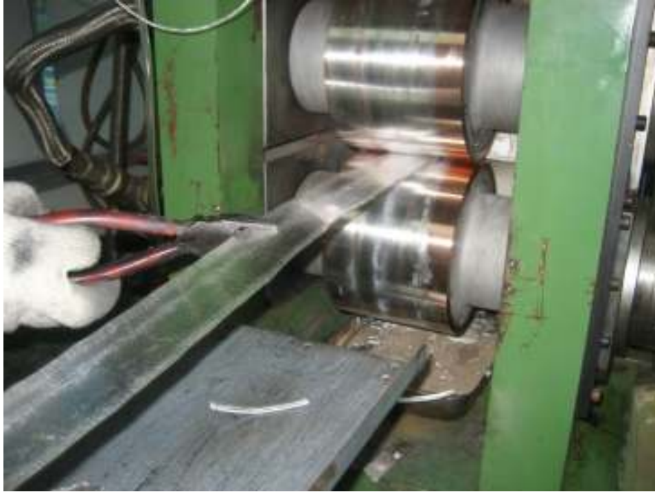
Figure 65 - Guiding the cast out of the rolls while removing any debris attached to the rolls
