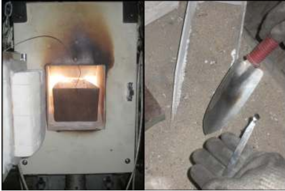
Figure 66 - Removing the tundish from the furnace and submerging it in sand
