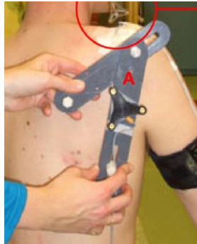
Figure 8: The scapular locator used in combinations with an active motion recording system (van Andel et al., 2009).
