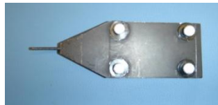
Figure 11: Stylus with four reflective markers.
