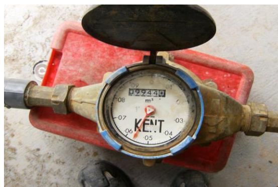
Figure D.9: Gauge used to measure flow rate and volume injected.
