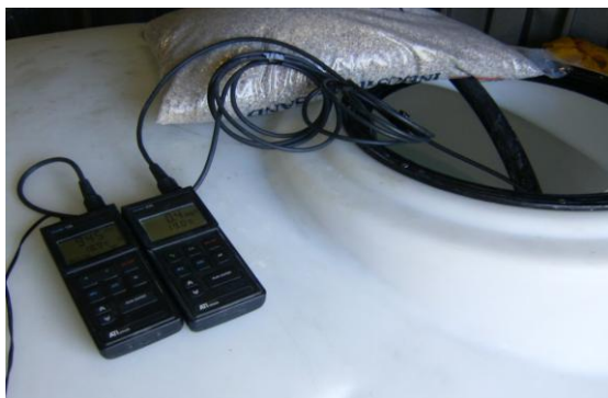
Figure D.7: Test solution anoxic following 1 hr N 2 sparging.
