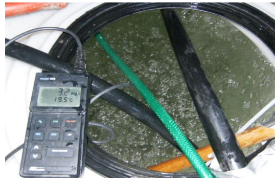
Figure D.6: Sparging test solution with N 2 to lower O 2 < 1 mg/L
