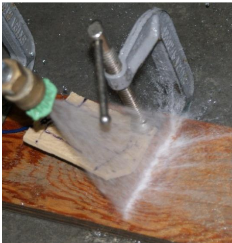
Figure 3.6. Photo of fibre glass coupon being power washed.
