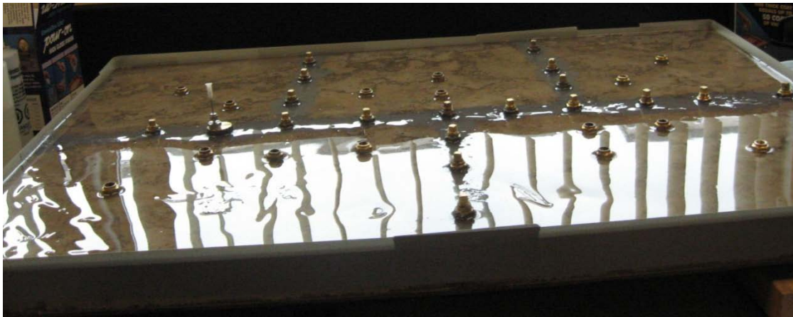
Figure 2.5: Photograph of the Fractured Rock Block Covered with Resin
