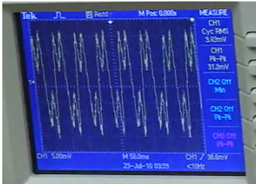
Figure 3.13: Output peak-to-peak voltage waveform from the harvester captured on oscilloscope
