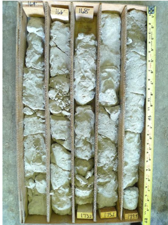
Figure A.7: Core photographs of CHAM-07-04A of the Glasford deglacial unit composed of repeated facies assemblage C and B.
