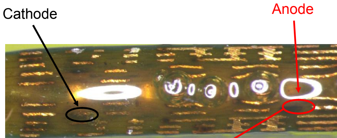
Figure 4-31: Optical image of test coupon B116 shorted at t_B = 180 hrs
