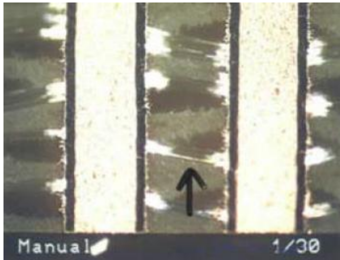
Figure 2-10: Copper wicking due to mechanical drilling [27 and 29]
