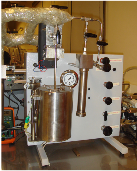
Fig. 6-1 A Sieverts-type apparatus custom-built by A.O.C. Scientific Engineering Pty Ltd., Australia, for evaluating hydrogen storage properties
