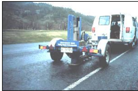
Figure 4-3. Falling Weight Deflectometer.
