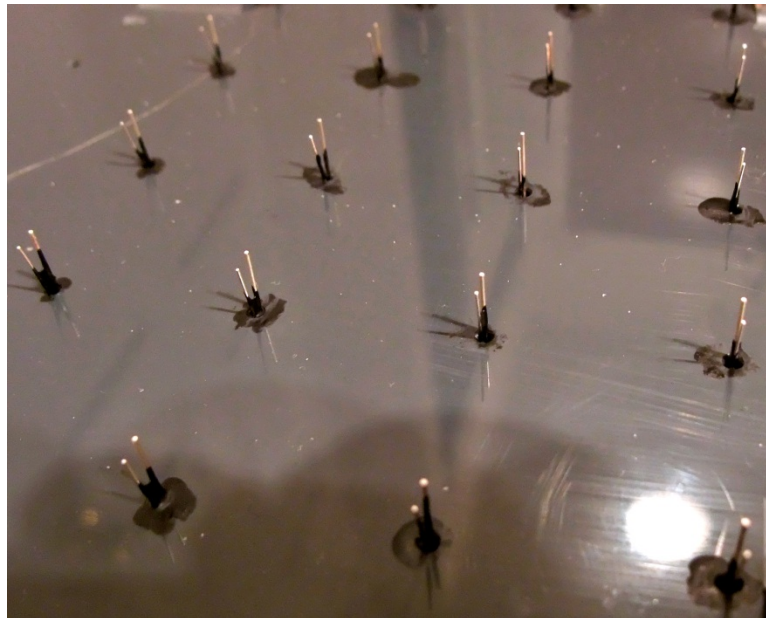
Figure 7.3. Close-up of the LED leads coated with liquid electrical tape.
