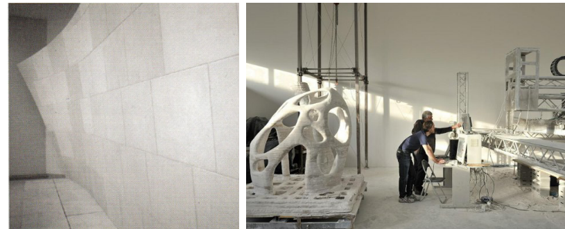
Figure 2.1-7 Gehry Partners experimented with custom-milled masonry for the Walt Disney Concert Hall (left). In the future, additive fabrication processes, such as Enrico Dini's masonry “printing” machine (right) may allow designers to create large and complexly shaped masonry units without the need for milling or molding.
