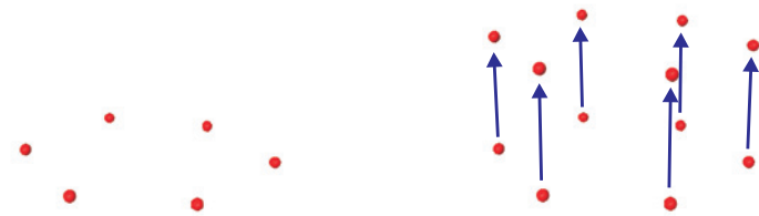
Figure 4.3-2 Step 1: Create a series of points on the XY plane and copy them upwards.
