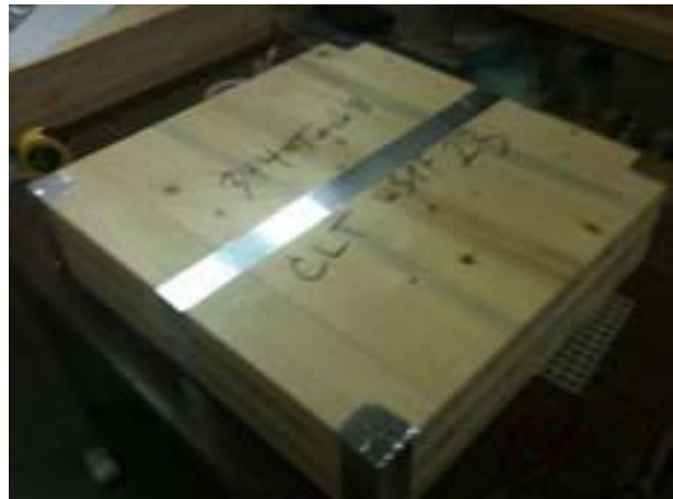
Step 2- Apply Al Tape along Joint
