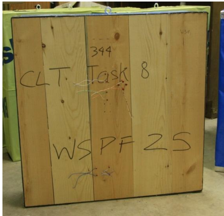
Figure 4.11: Fully Prepared CLT Sample
