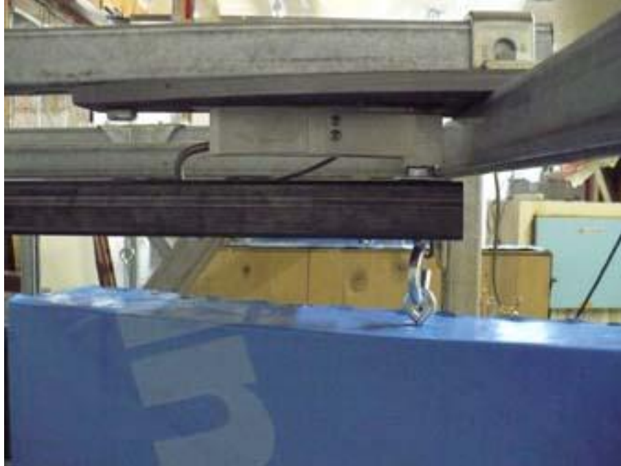
Figure 4.6: Five-Pound Capacity Beam-Type Load Cell
