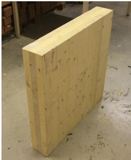
Figure 2.1: 3-Ply CLT Panel Sample
