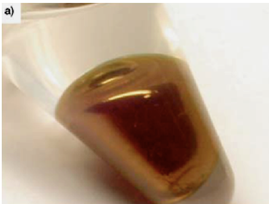
Figure 2.10: Image of the self-assembled Au@DTBE nanoparticles at the water/toluene interface in a plastic tube [69].
