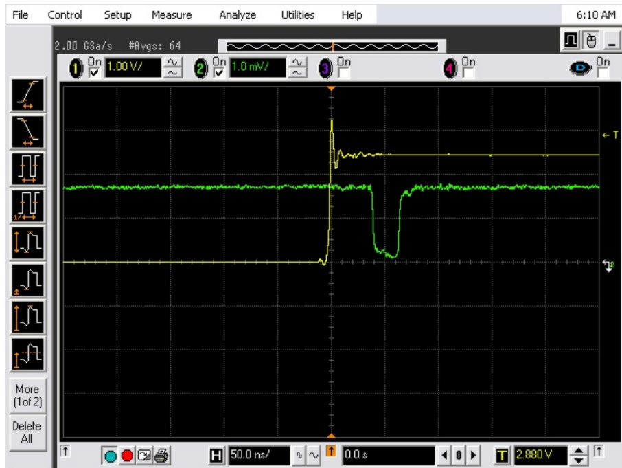
Figure 5.3: The figure shows the oscilloscope trace measured while finding the PC halfwave voltage (HWV). The PC was operated between a parallel polarizer and PBS set to transmit and project on H polarized photons. Photons were measured with a fast photodiode. The PC was triggered at a repetition rate of 30 kHz with a function generator and accompanying splitter box as the high voltage power supply was slowly adjusted. The HWV was found as the setting which minimized the trace during the time when the PC was on corresponding to the PC rotating the incoming photons by 90^\circ to V. The yellow trace was the sync signal from the function generator while the green trace was the output of the fast photodiode.
