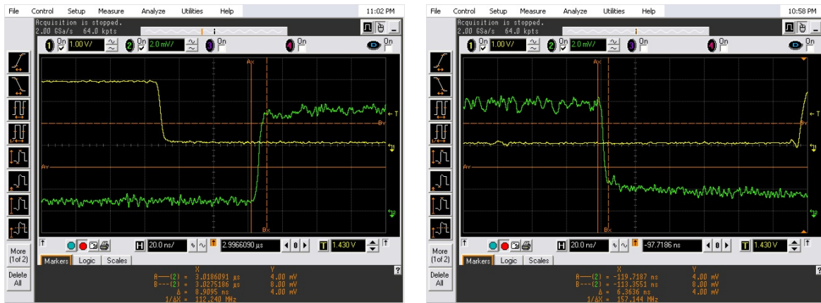
Figure 5.5: The figure shows the oscilloscope trace measuring the (left) rise time and (right) fall time of the PC as it was triggered at a rate of 0.956 MHz with a minimum pulse length of 1 \mu s. A rise time of 8.9 ns and a fall time of 6.4 ns were measured at the QWV leading to a duty cycle of 98.40%. The green trace is the signal from the fast photodiode, while the yellow trace is the state of the PC.
