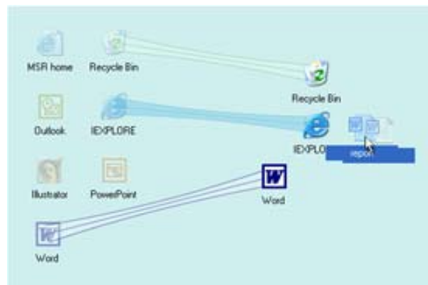
Figure 2.5: Baudisch et al.'s Drag-and-pop [5] technique. Virtual proxies of icons on the far left of the screen are brought closer to the cursor to facilitate quick pointing by reducing A . The relationship between proxy and actual icon is indicated by the stretched lines. The proxies only exist for the duration of the cursor drag action, thus not affecting the overall interface. Adapted from [5].
