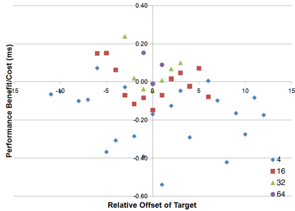
Figure 7.7: Performance Benefit/Cost by relative displacement of a user’s target for targets of size 4, 16, 32, and 64-pixels for the correct experimental condition.
