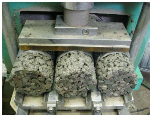
Figure 3-5: Cylinder Sample End Preparation by End Grinding
