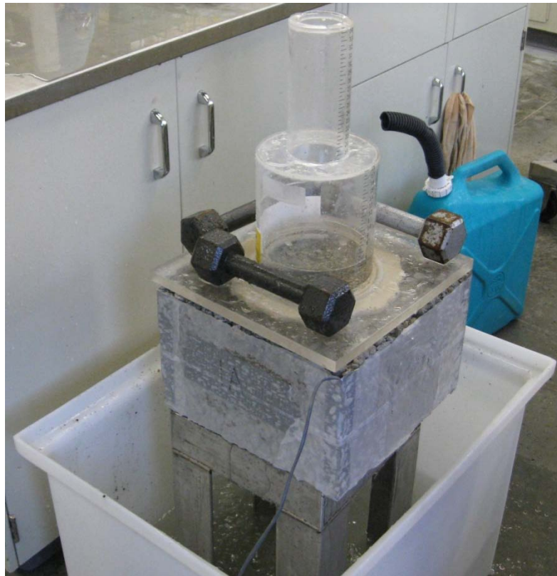
Figure 3-9: Permeability Testing of a Slab in the Laboratory
