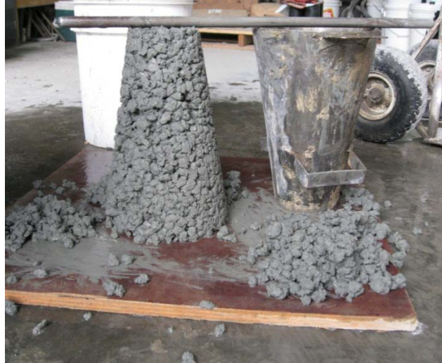
Figure 3-2: Measuring the Slump of Pervious Concrete
