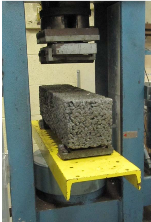
Figure 3-6: Flexural Beam in Testing Frame
