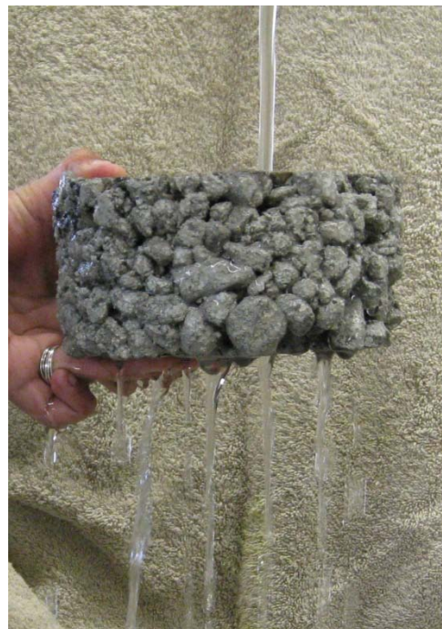
Figure 1-3: Pervious Concrete Pavement
