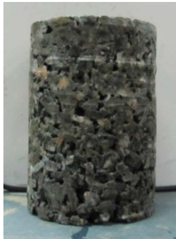
Figure 5-1: Varying Density in a Core from Site 5
