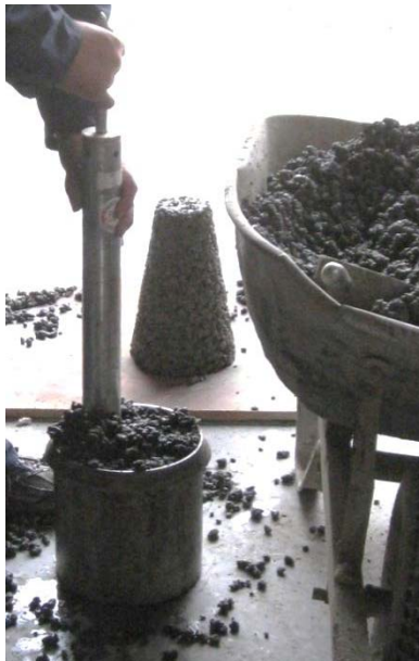
Figure 3-4: Proctor Hammer Compacting Pervious Concrete for Density Testing
