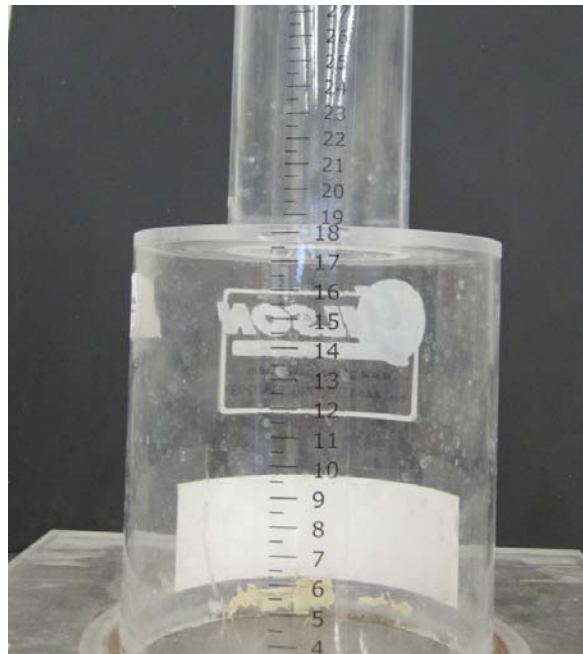
Figure 3-8: Graduated Measurement Markings on Permeameter
