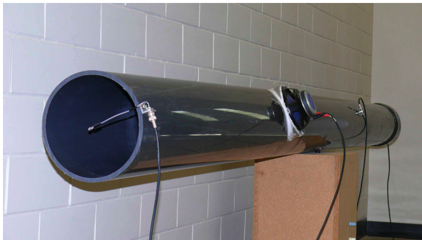
Figure 1.2: Acoustic noise in a duct [96, Fig. 2]: A noise signal is produced by a loudspeaker placed at one end of the duct. An actuator loudspeaker is mounted midway down the duct to control the noise signal.
