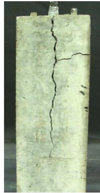
b) Post-failure cracking
