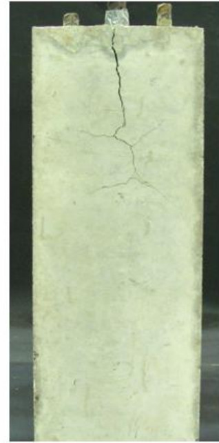
b) Post-failure cracking
