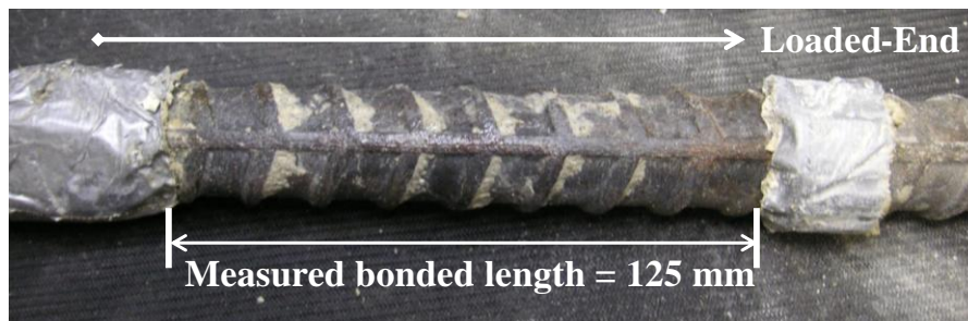
Figure 9.33 Main test bar, measured bonded length and adhered concrete (dissected BE-RAC2-30-125B)
