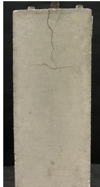
b) Post-failure cracking
