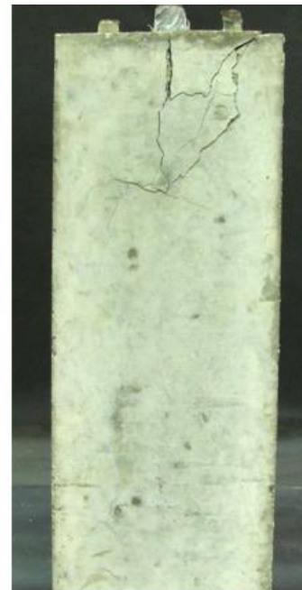
b) Post-failure cracking
