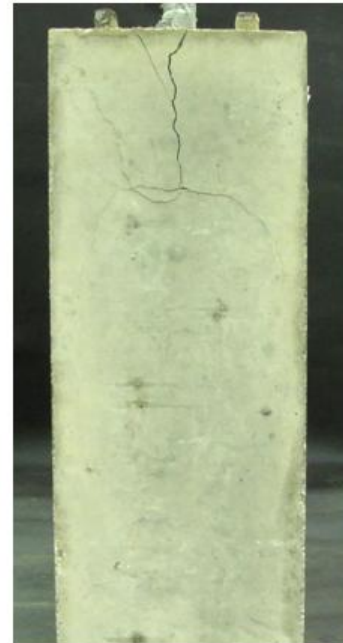
b) Post-failure cracking
