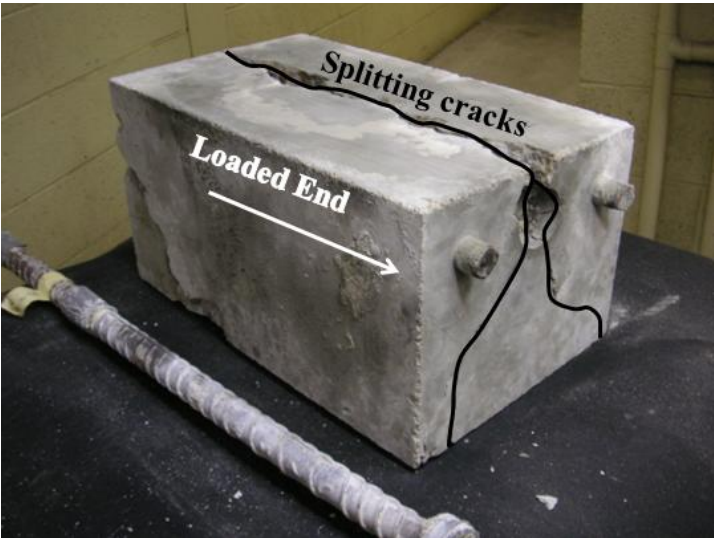
Figure 9.25 Main anchorage zone and splitting crack pattern (dissected BE-NAC-50-375A)
