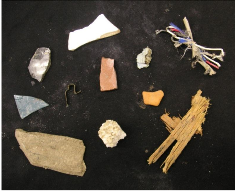
Figure 4.2 Deleterious materials present within RCA-2
