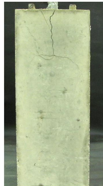
Figure D.25 Bond-slip response and crack pattern for BE-NAC-40-125A
