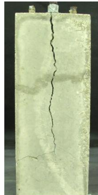
b) Post-failure cracking
