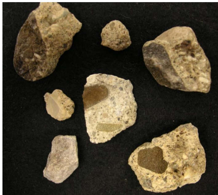
Figure 4.5 RCA-1 old adhered mortar and original aggregates
