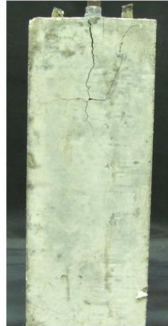
b) Post-failure cracking
