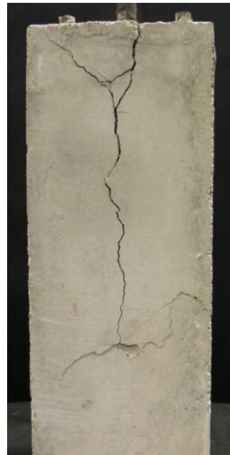
b) Post-failure cracking
