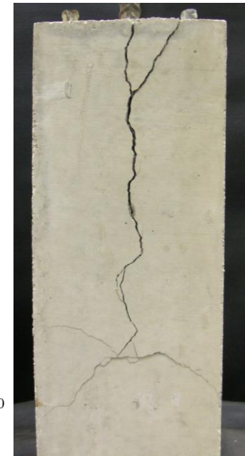
b) Post-failure cracking
