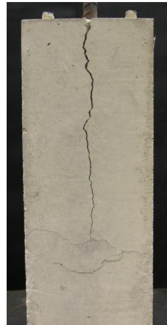
b) Post-failure cracking
