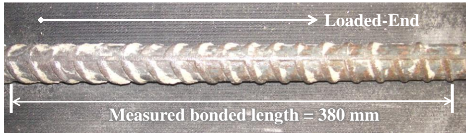
Figure 9.30 Main test bar, measured bonded length, and adhered concrete (dissected BE-RAC1-30-375A)
