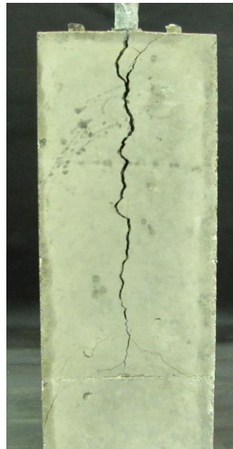
b) Post-failure cracking
