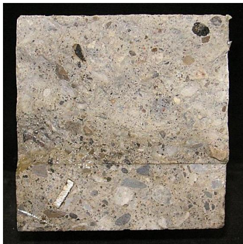
Figure 8.16 Fracture zones of fracture energy prisms (Phase 1 30 MPa specimens)
