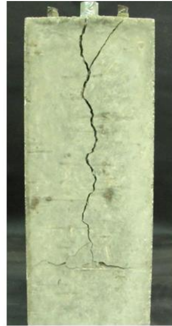
b) Post-failure cracking
