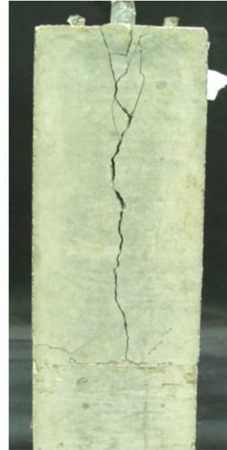
b) Post-failure cracking
