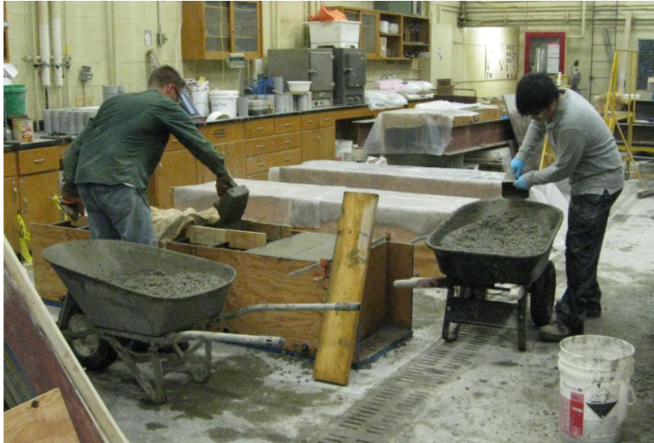
Figure 9.6 Beam-end casting and curing techniques
