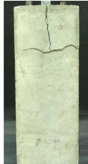
b) Post-failure cracking
