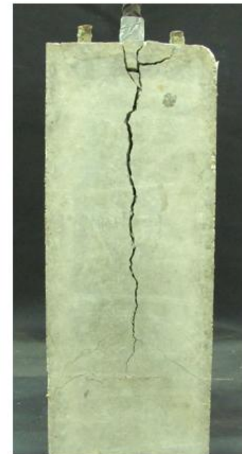
b) Post-failure cracking
