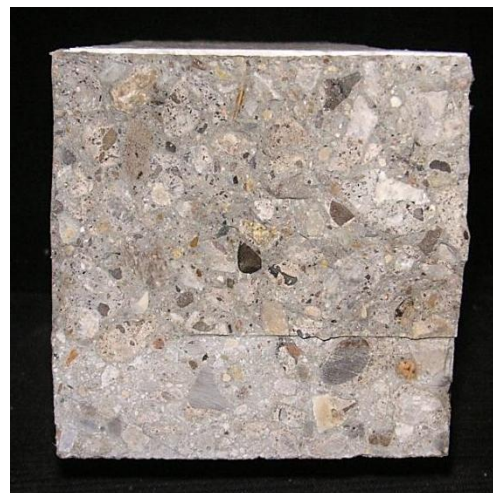
Figure 8.17 Fracture zones of fracture energy prisms (Phase 1 50 MPa specimens)
