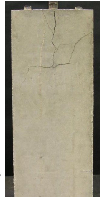
b) Post-failure cracking
