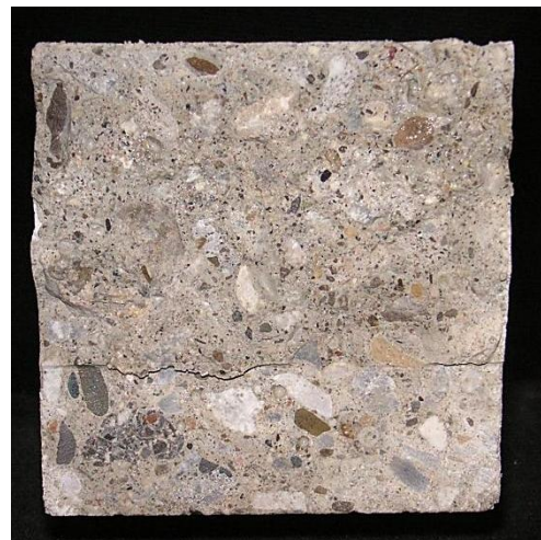
Figure 8.16 Fracture zones of fracture energy prisms (Phase 1 30 MPa specimens)
