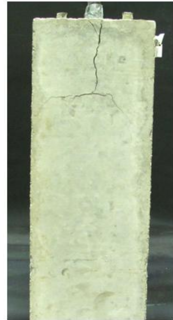
b) Post-failure cracking
