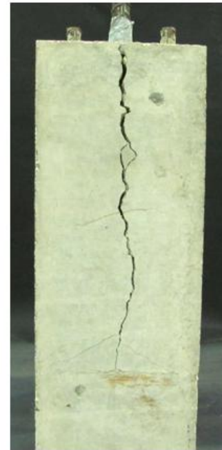
b) Post-failure cracking
