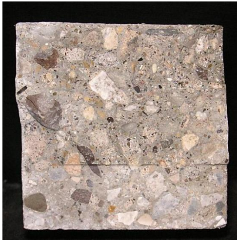
Figure 8.17 Fracture zones of fracture energy prisms (Phase 1 50 MPa specimens)
