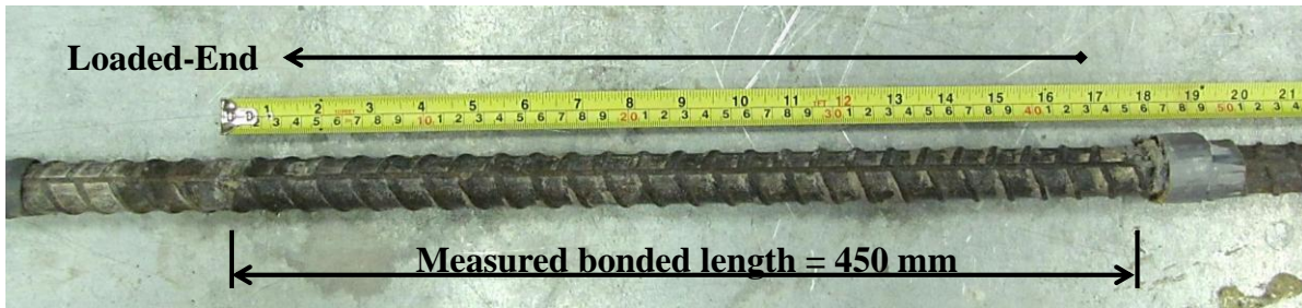
Figure 9.53 Main test bar, measured bonded length, and adhered concrete (dissected BE-NAC-40-450B)
