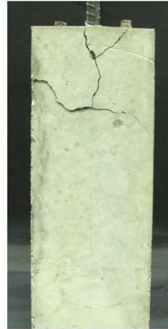
b) Post-failure cracking
