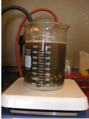
Figure 4.6 Heating of RCA in nitric acid bath
